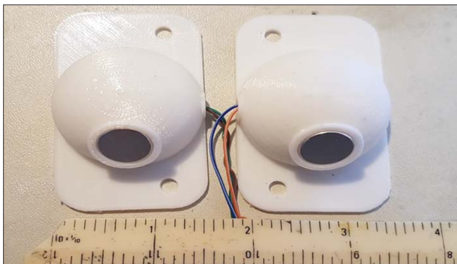
The ultrasound transmitter and receiver. These little devices make no physical contact with the train, but detect a signal reflected off the wheels and other parts. The housings are 3D printed PLA plastic
