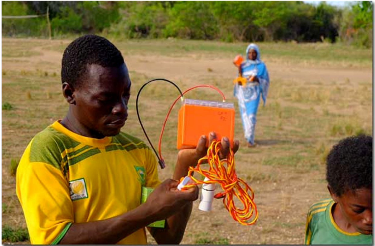
Portable power – a 12 V motorcycle battery, LED fixture, and wiring for household use. (Photo: Jeff Schnurr)
