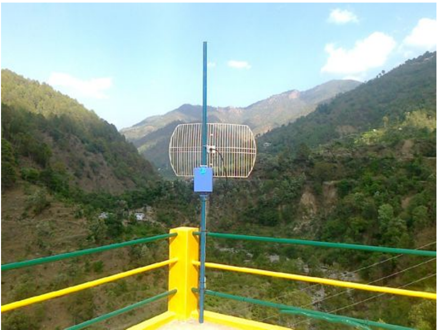
Figure CSD 10: Client Relay, Kangra Valley Network
