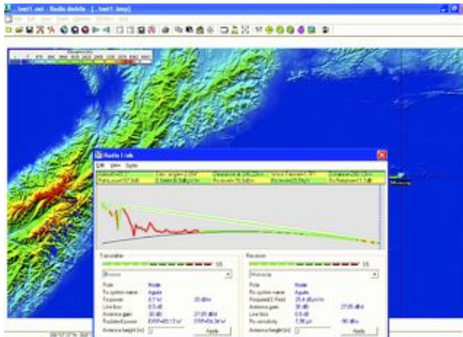
Figure OI 3: Profile of a 280 km path over which standard WiFi gear with OpenWRT firmware which allows for the ACKtimeout increase was used to transfer files at about 65 kbps in April 2006 between Pico del Aguila and El Baul in Venezuela.
