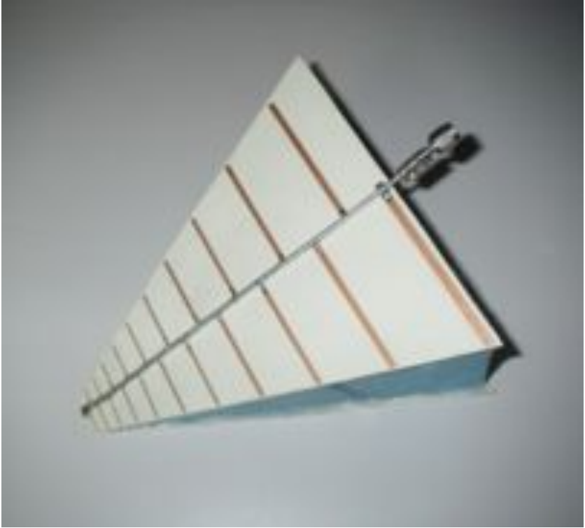
Figure ATL 16: Log periodic antenna
