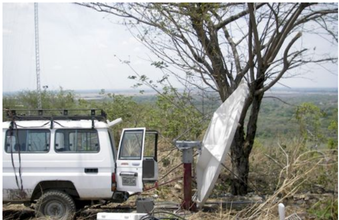
Figure CsLD 9: El Baúl antenna installation. Actual elevation was 1° upward, since the antenna has an offset of 22.5°.
