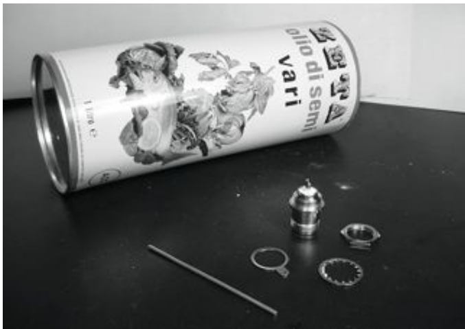
Figure AC 21: Parts needed for the cantenna.
