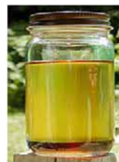
Figure 6. Biodiesel and glycerol after transesterification
