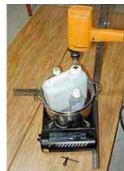
Figure 5. Assembly kit for transesterification
