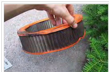
Auto engine air filter clogged with dust and grime
