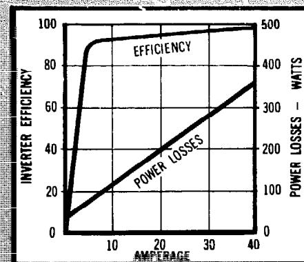
In addition to minimizing system losses associated with current level, operating at higher voltages results in a minimum V/AF load imposed on the AC lines.
