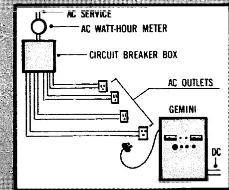
Three phase units can be wired in permanently to the circuit breaker box serving the AC loads or facility in question. For both single phase and three phase applications the Gemini should be isolated on its own circuit and circuit breaker. Power from the DC source is then fed through the Gemini to the circuit breaker box where it is automatically distributed to any AC loads or fed back to the AC source.
