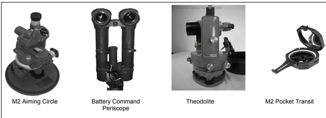
**Figure G-1. Unit Organic Optical Equipment Ideal for Sighting Measurements**
