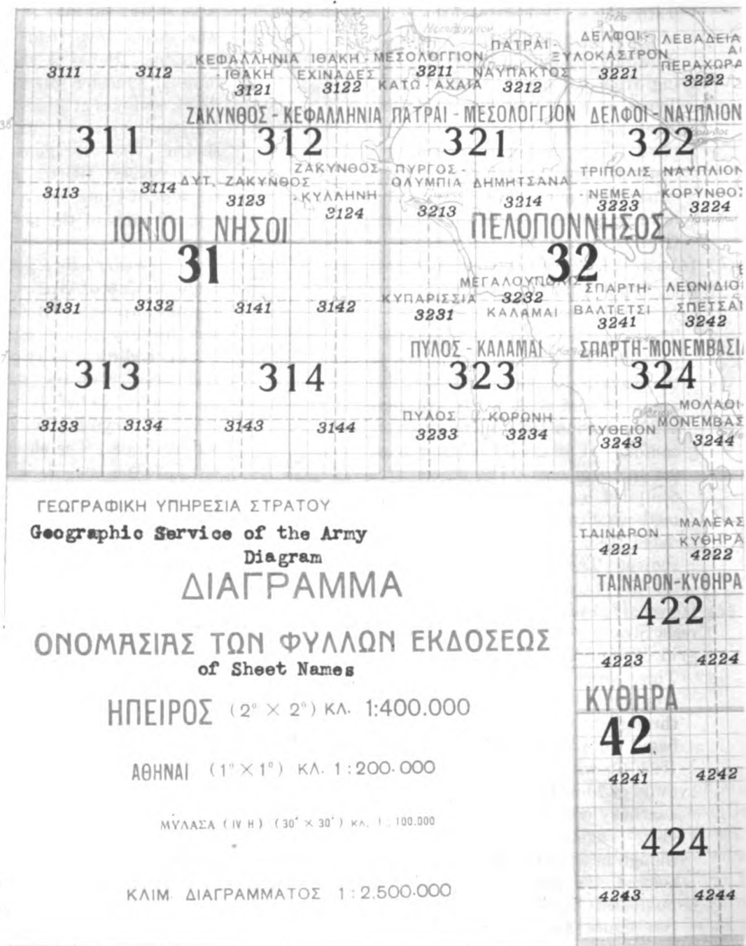
Figure 140. Section of Greek index illustrating sheet-line system of maps published by the Yeografiki Ipiresia Stratoú.
