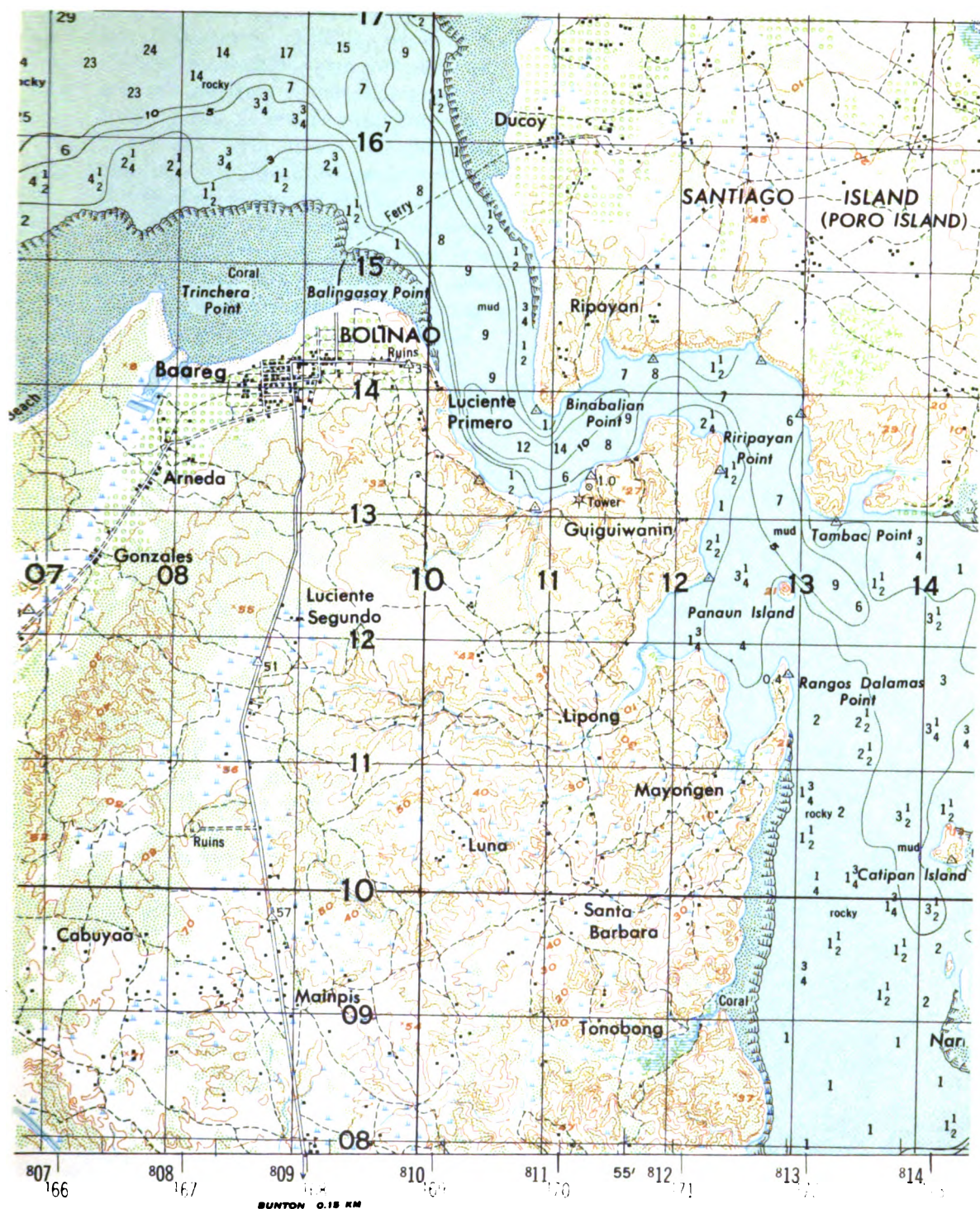
Figure 93. Section of sheet from the Luzon 1:50,000 series (AMS S711), by the 64th Engineer Base Topographic Battalion.
