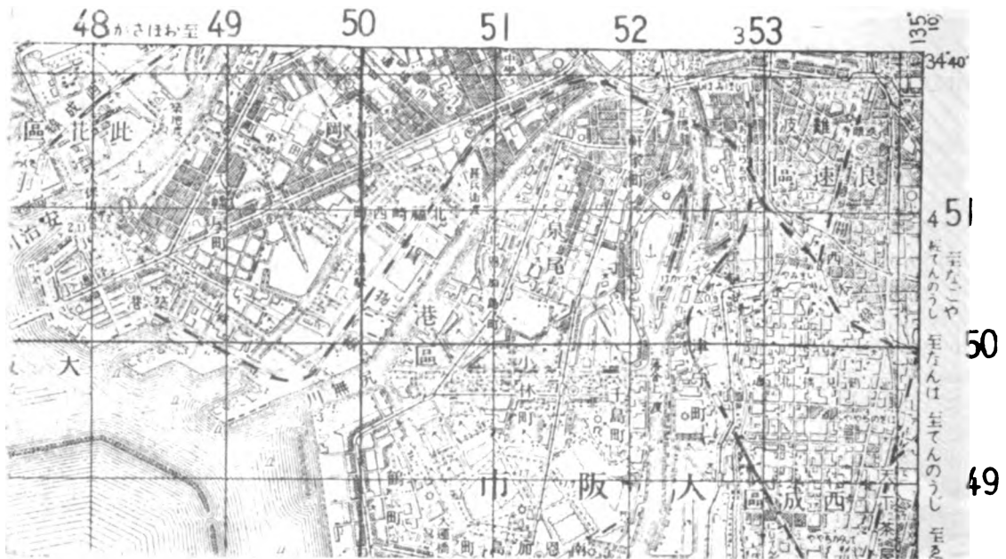
Figure 45. Section of sheet (Osaka) from oversized Japanese 1:50,000 series with Gauss-Schreiber type grid.
