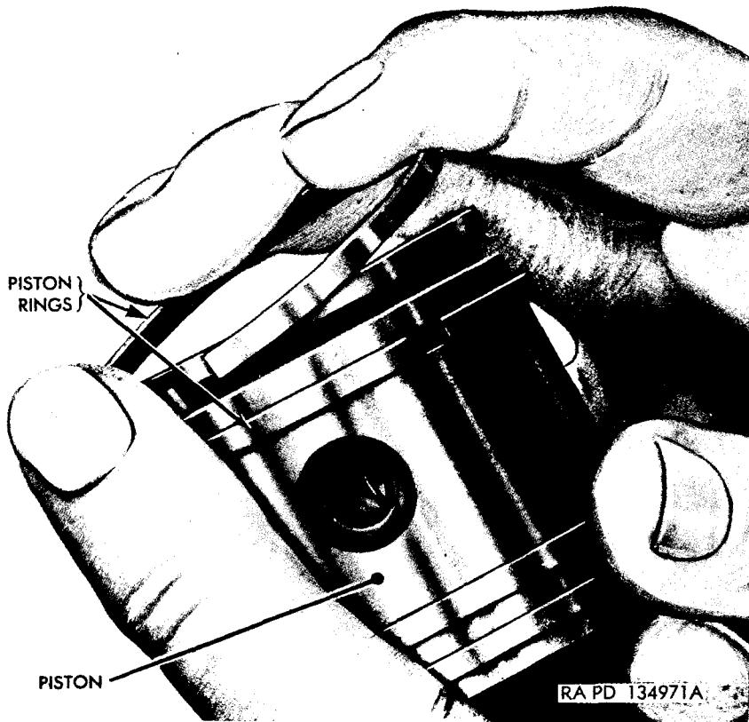
Figure 50. *Installing piston rings.*
