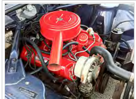
Alternator (silver) mounted on a V8 engine
