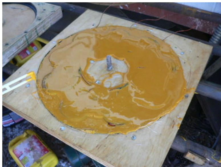
Then fill the mold with resin and be sure all surfaces of the coils have resin on them.
