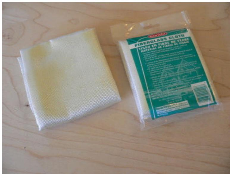
The stator will be cast in the same polyester resin you used for the magnet rotors. You'll need fiberglass cloth on both sides of the coils. It might be useful to review the section on casting magnet rotors before doing this as the procedure is very similar and safety precautions are the same.
