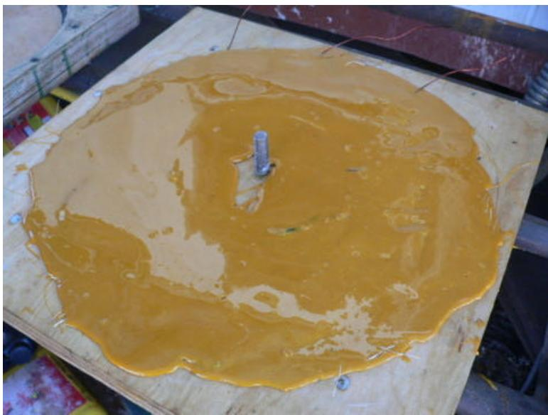
Pour the remaining resin over the top of the fabric. Work it in and try to work out air bubbles. It might not hurt at this time to beat on the mold a bit or vibrate it with a sander (or something) for a couple minutes to help air bubbles rise to the top.
