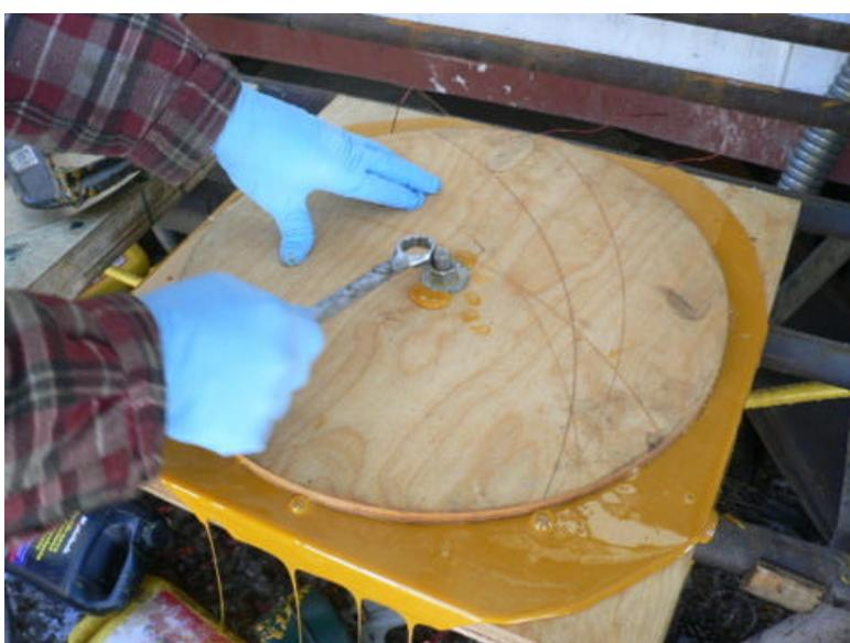
Put a 1/2" washer over the threaded rod, and run the 1/2" nut down over it. Tighten the nut - this does a good job of clamping the lid tightly on the mold and assuring that the finished casting will be 1/2" thick.
