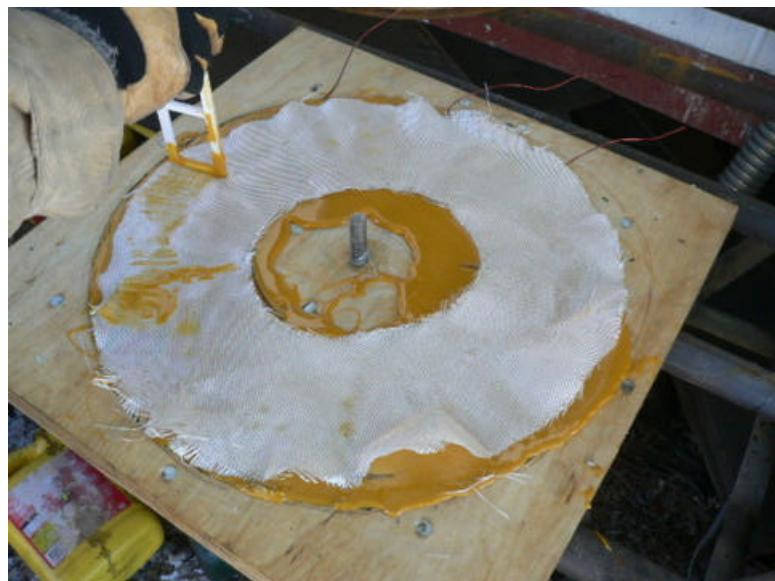
Put the remaining fiberglass ring over the top of the coils and work resin into it - again, it should almost disappear.
