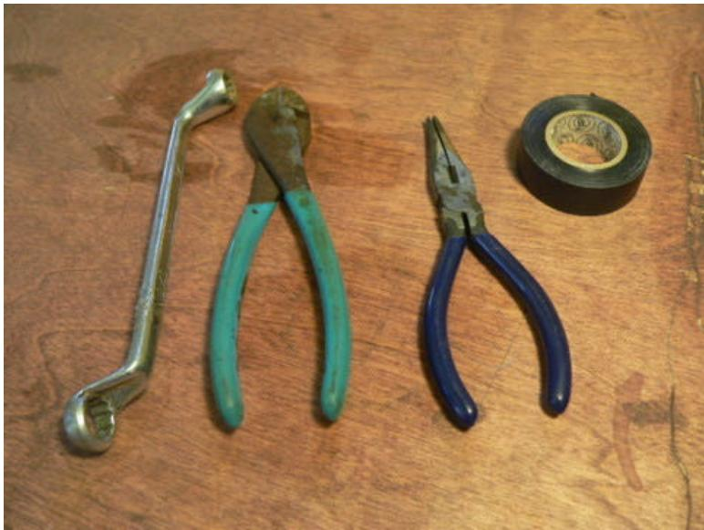
You'll need a pair of side cutters (to cut the wire), a pair of needle nosed pliers (to bend the wire) and some electrical tape. If the coil winder has a wing nut holding it together then you can use your fingers to take it apart. Otherwise you'll need a 1/2 wrench. When you bolt the front on the coil winder finger tight is fine, but after all the wire is wound on the spool the nut will be tight so - if you dont have a wing nut, you'll need a wrench to get it apart.
