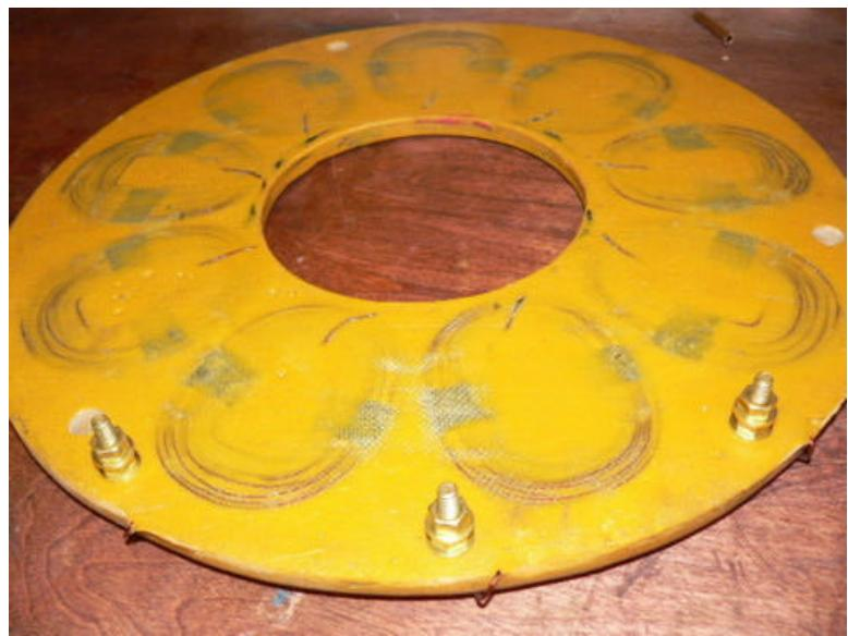
The stator is finished! We can put that aside until we're ready to assemble the alternator.
