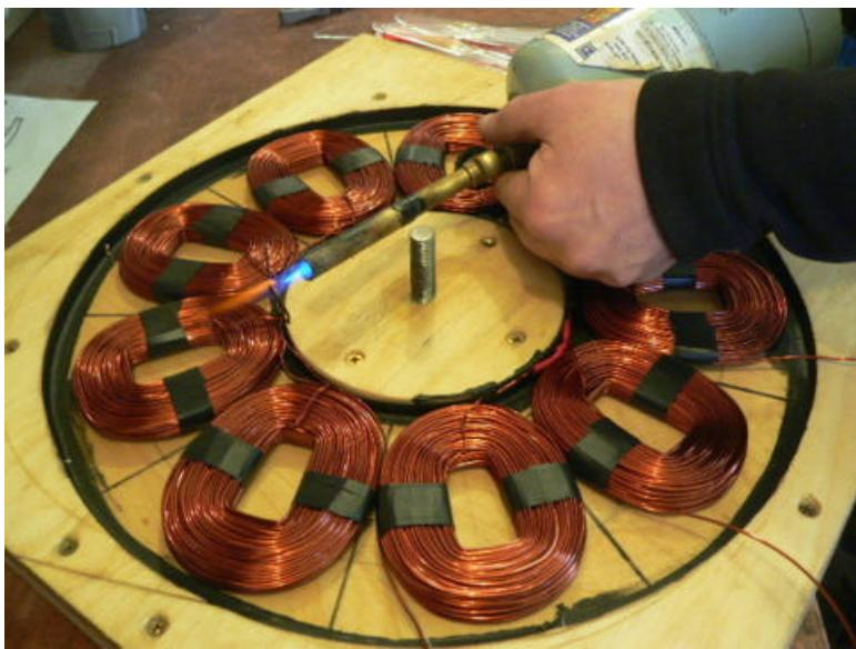
Now you need to make the star connection between the phases. The 3 inside leads should be brought together so that we can connect them together. Leave enough slack in the wires so that we can make this connection, and then push it down between the coils and the island in the mold. So figure the length, cut them off, burn the insulation with the torch, sand it, twist them and solder them. Then insulate the connection with electrical tape or heat shrink.
