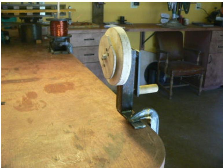
Clamp the coil winder to the workbench with a C clamp as shown in the picture.
