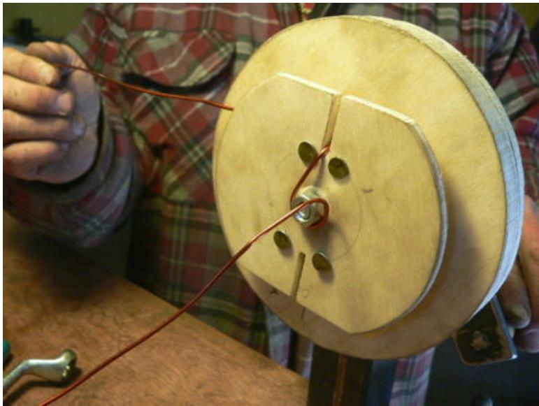
Drop the wire in the slot of the coil winder and bend the end around the nut. (A wing nut helps here too..) This will hold the wire from slipping when you wind the coil.
