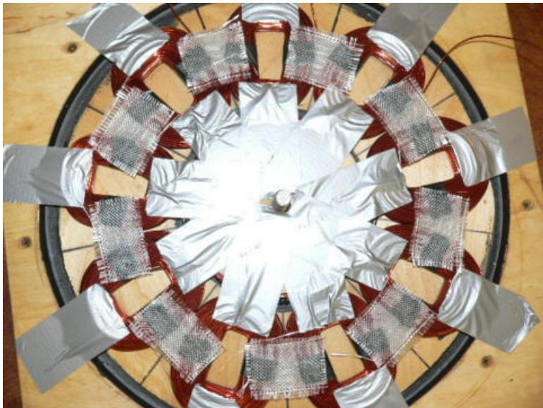
In the picture you can see all the coils are connected to one another with fiberglass cloth.
