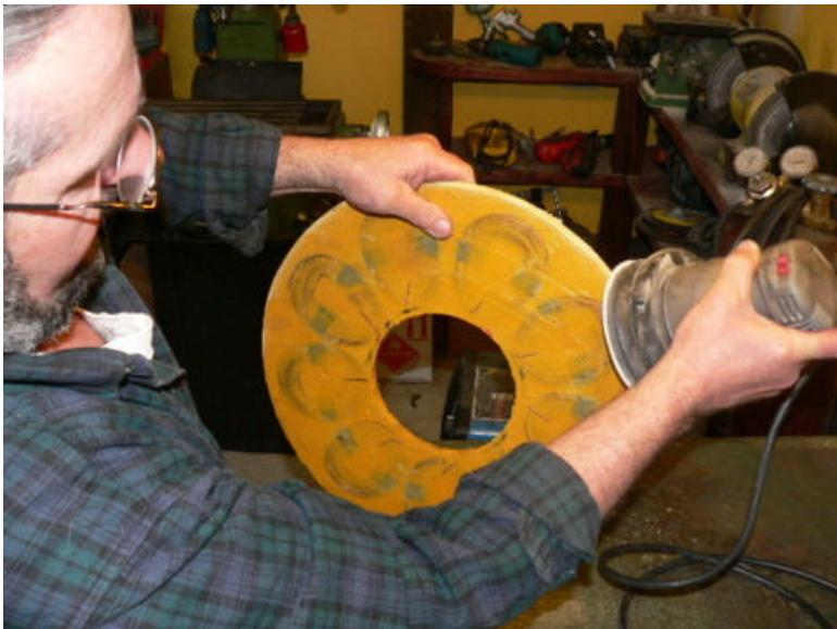
Use a file or a sander (or both) to clean up the edges of the stator. The inside diameter must be pretty clean because there's not a lot of extra room between this hole and the wheel hub which will exist inside it.
