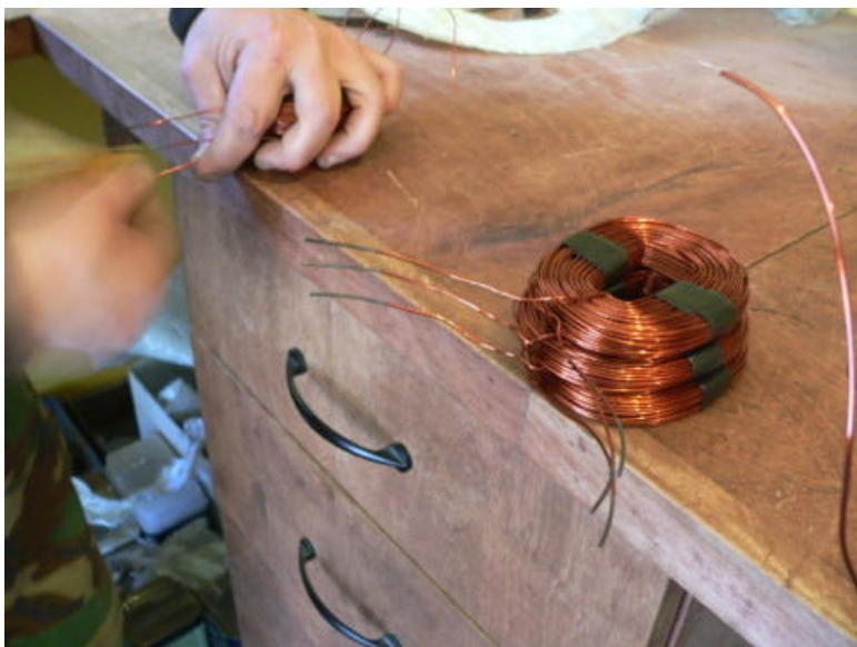
Let the wires cool down, and then clean the burned insulation off carefully with sand paper.
