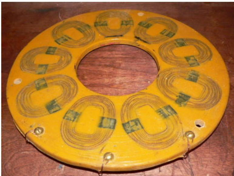
Insert a brass 1/4 - 20tpi screw through each one, with a washer on each side and a nut on the back. Cut the leads just long enough so you can clamp each one between a screw head and the washer. You can put a couple more washers and one nut on each screw now. These will serve as the lugs to which we can connect the line to the wind turbine.
