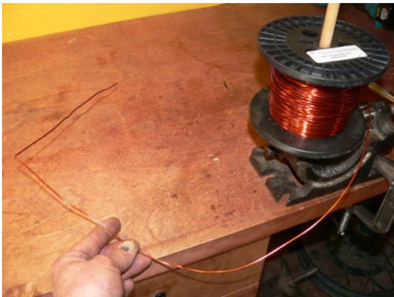
About 10" from the end of the wire bend it sharply 90 deg with the needle nosed pliers.
