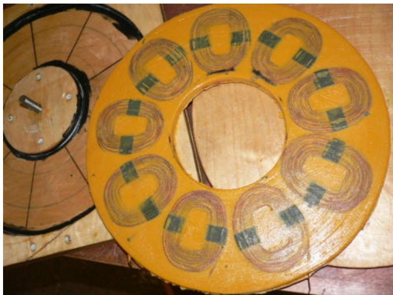
Once the lid comes off you can usually turn the mold upside down and the stator will just fall out. If not then turn the mold upside down and tap on it with a hammer or pry gently at the edge of the stator. It should come out easily.
