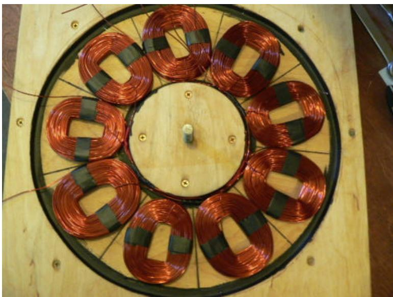
Once all three phase are finished, put all three back into the mold as shown in the picture. Do it such that your three 'ends' (those wires that are pointing towards the outside of the mold) are beside each other. Those three 'ends' will be the leads out of the stator (the output from the wind turbine).
