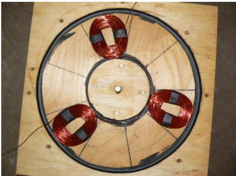
Put the 3 coils back in the mold and twist the wires together tightly. You can see in the picture how the connections are pretty much centered in between the coils. Then solder the connections, and bend them over with pliers so you can insulate them with electrical tape and keep it all as thin as possible. You can also use heat shrink here for neater appearance - if you do, be sure to put that on before you twist the leads together!
