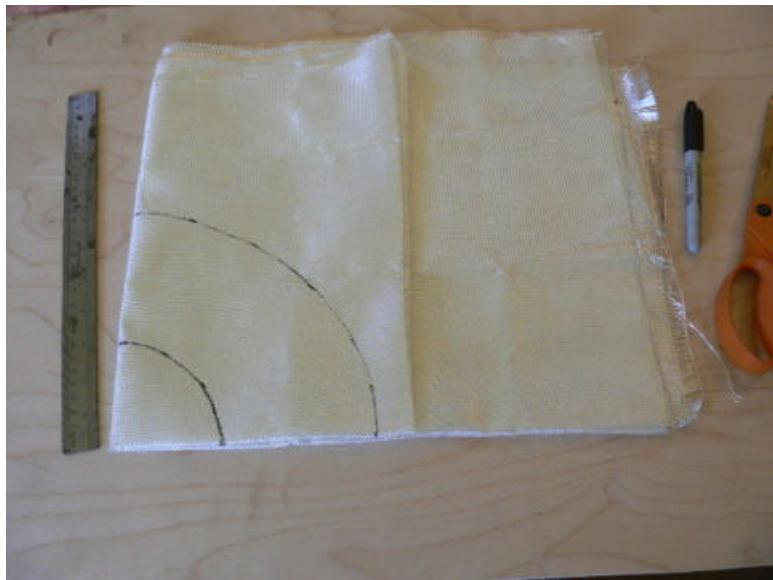
If you fold the fabric correctly, you can lay out just 1/4 of the ring and cut out two in one shot. You need two rings of fiberglass 15" outer diameter and 6" inner diameter.
