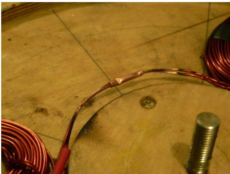
If you're building a 12 Volt machine with multiple strands of wire it can be tricky to twist things together nicely. For machines that have multiple strands, it works well to make your connections by inserting the coil leads into small copper, or brass tubing - and then crimp and solder.
