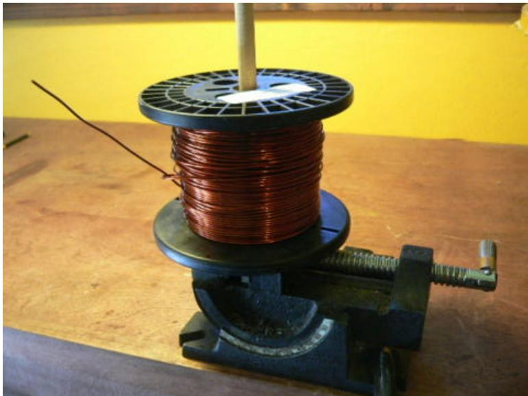
Start by creating some kind of fixture to hold the spool of magnet wire. I usually use a vice with a piece of threaded rod, or a wooden dowel sticking up to put the spool. Clamp it to the work bench securely.
