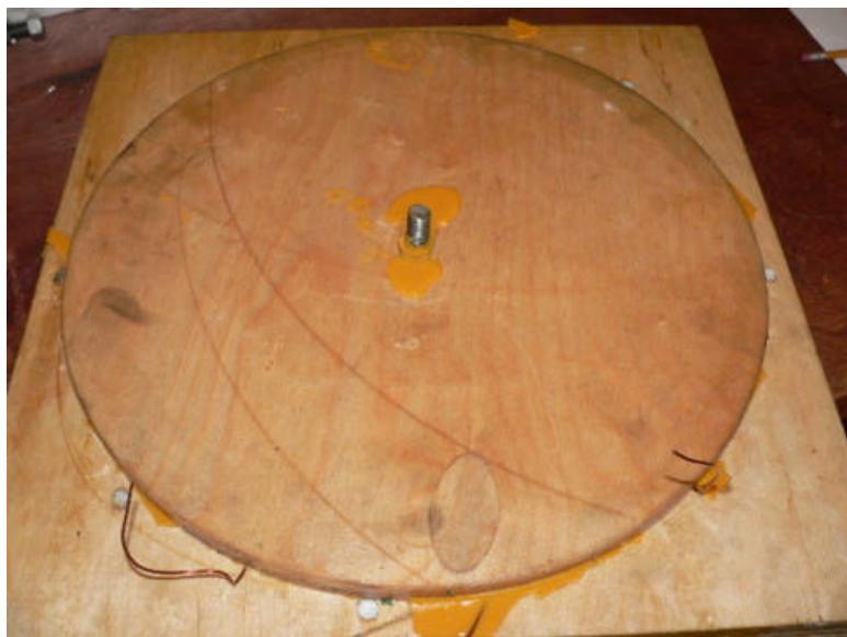
Once the resin seems hard then remove the C clamps and the nut in the center. Use a chisel or a screw driver to gently pry around the lid until it breaks loose.
