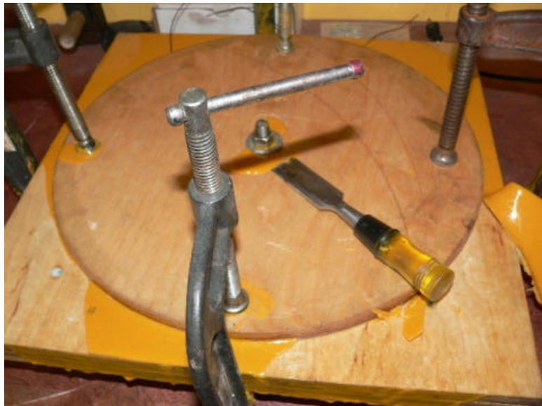
A chisel works well to scrape/peel the resin off around the outside of the mold. A good time to do this is while it's still a bit flexible (before it gets really hard).
