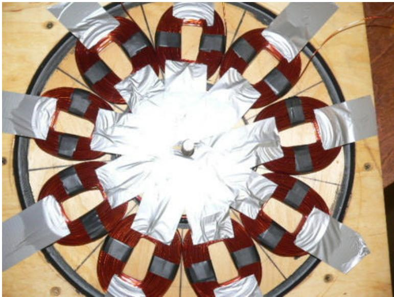
Even though the coils fit well and are the right size, once we make all these connections things are kind of springy and surely the coils are not in their perfect place. The connections we made and all that wire around the inside is sure to push some of the coils out further than they ought to be. Use duct tape and go around the stator 1 coil at a time, and tape it exactly where it belongs. Keep the tape off the 'legs' of the coils as shown in the picture.
