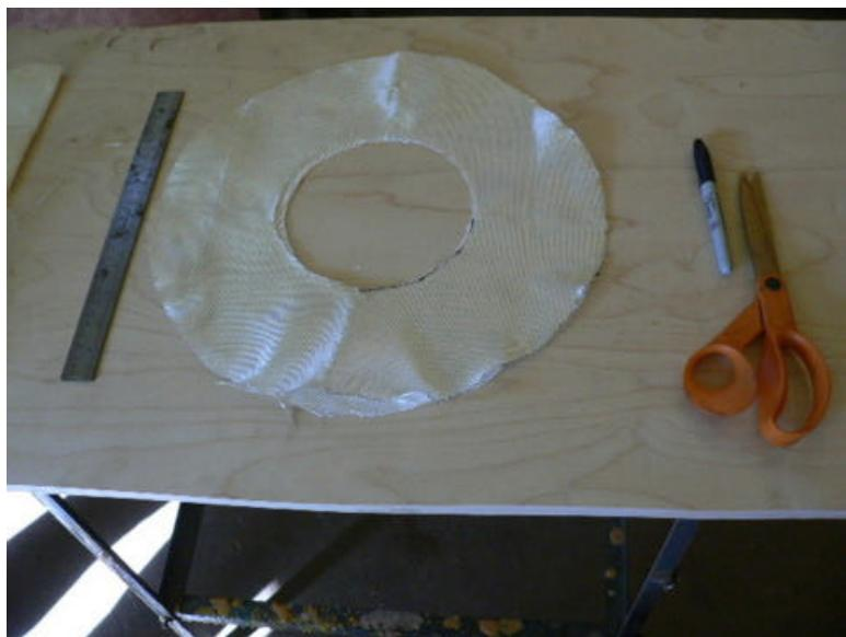
In the picture you can see the two rings of fiberglass. Set them, and the coils aside for now. Grease the stator mold inside, on top - and around the edge. Same with the lid - everything should be carefully covered with grease, or wax. Automotive or wood wax works really well.
