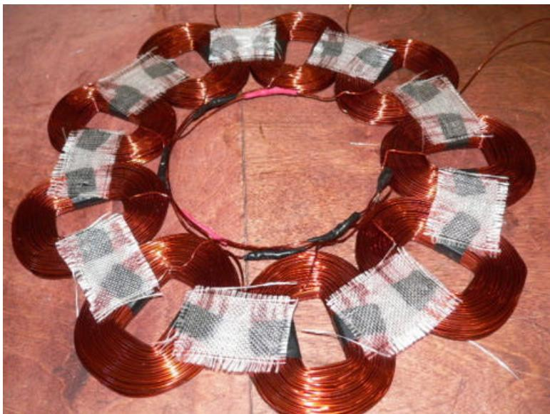
Now you can carefully pick up the uncast stator and remove it from the mold. Put it somewhere safe until you're ready to cast the stator in resin.
