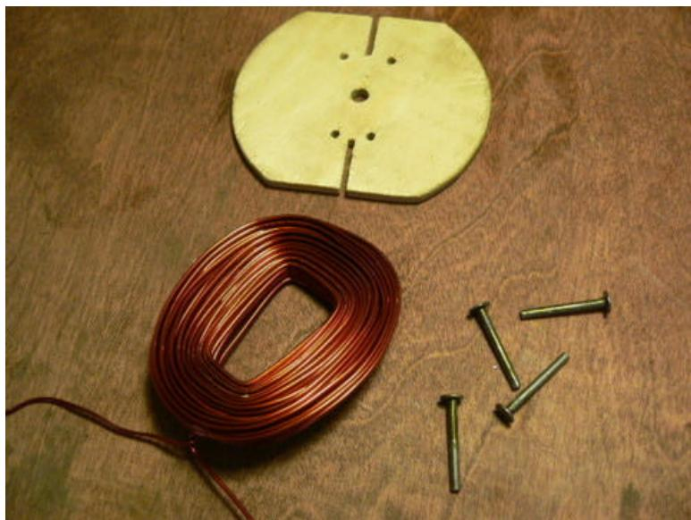
The coil should pretty much fall off the end if you just turn it over. Do it carefully so the coil doesn't fall apart.
