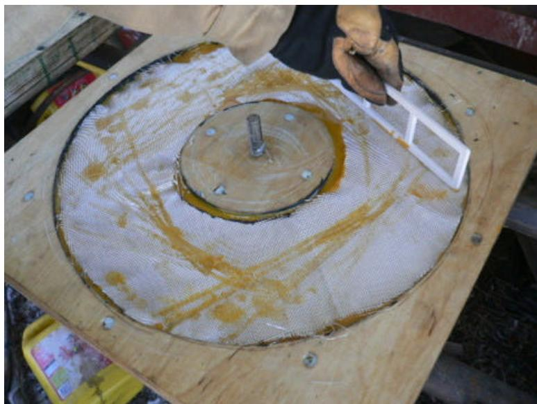
Put one of the fiberglass rings into the resin and work it with a stick until it becomes saturated. When saturated - the fabric will become almost invisible. (you won't see any white)
