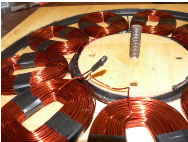
Pictured above is the finished star connection, all that needs to be done is to poke it down so it doesn't stick up above the coils.
