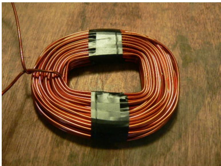
We refer to the longest sides of the coil as the 'legs'. Tape the legs of the coils with a couple wraps of electrical tape to hold things together. One coil is finished.
