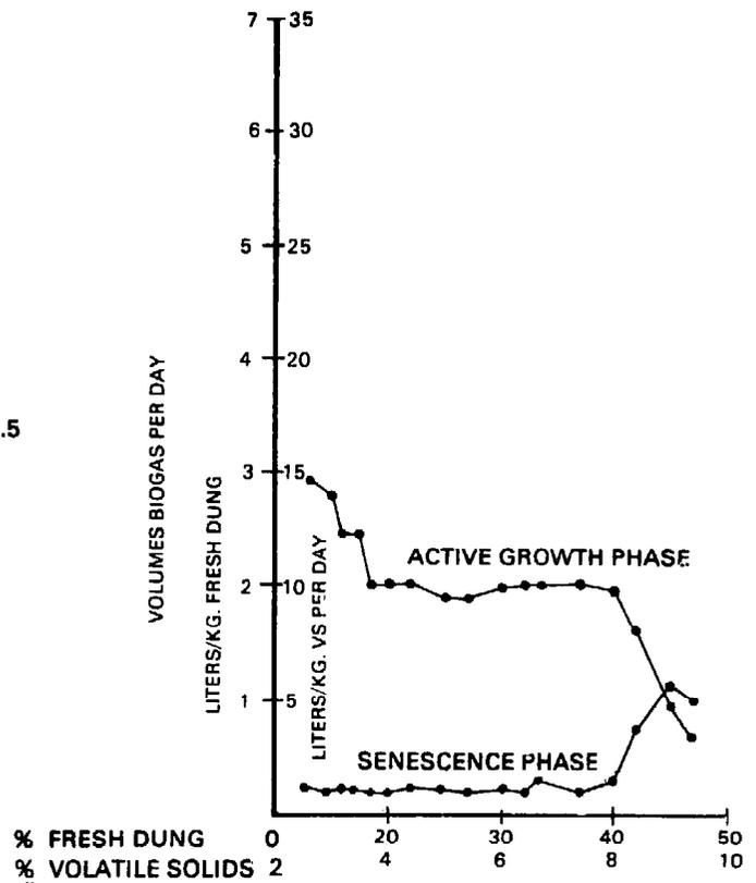
**FIG. 3-10 RATES OF BIOGAS PRODUCTION DURING ACTIVE GROWTH AND SENESCENCE IN RELATION TO DUNG CONCENTRATION.**
