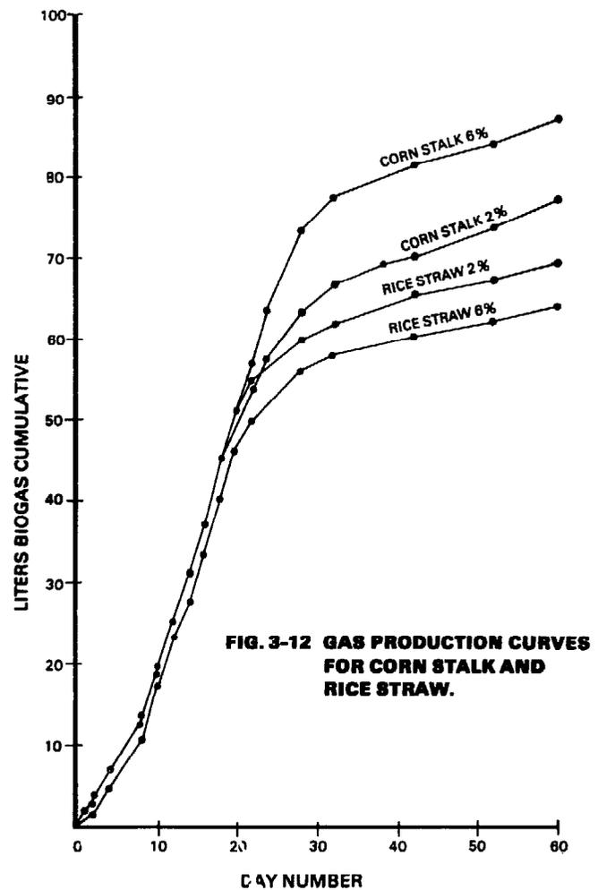
**FIG. 3-12 GAS PRODUCTION CURVES FOR CORN STALK AND RICE STRAW.**
