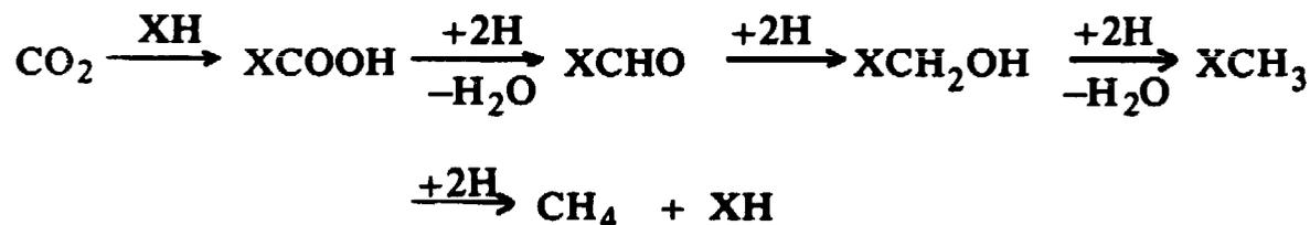
The hydrogen carrier is regenerated and recycled as illustrated above.
