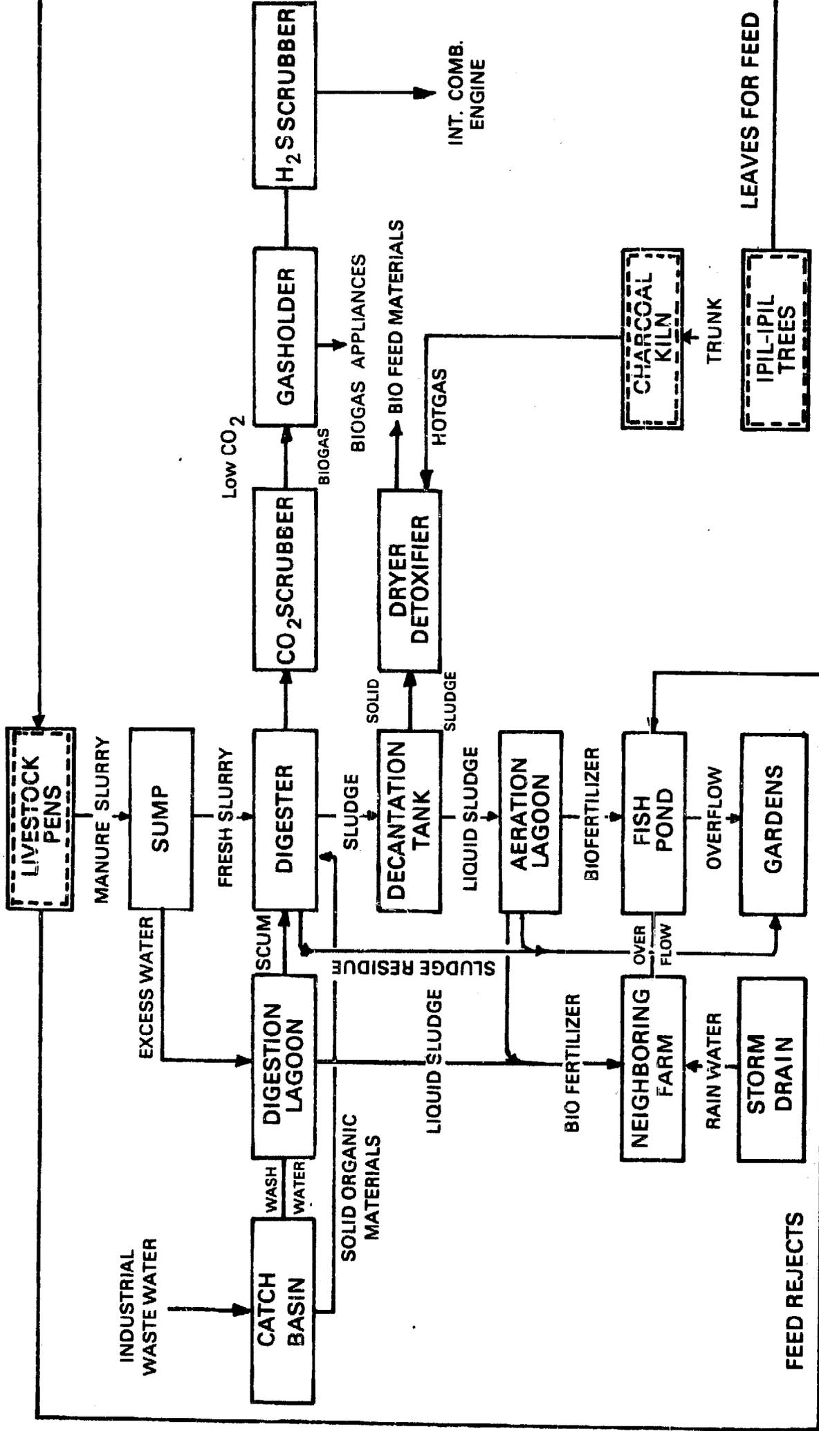
**FIG. 9-6 INTEGRATED MEAT PROCESSING BIOGAS WORKS FLOWSHEET**
