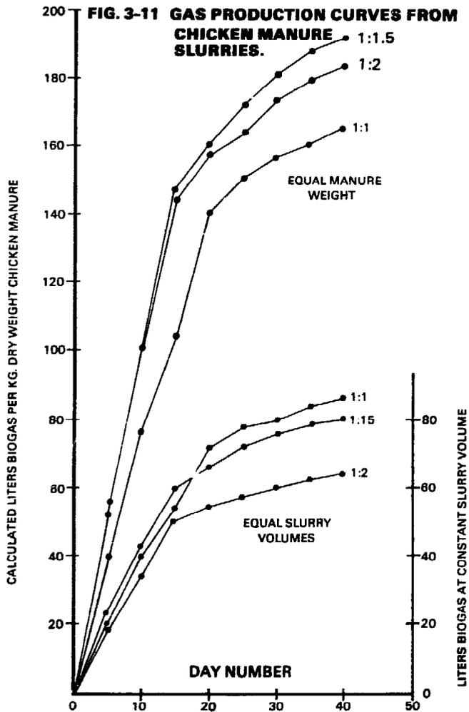
**FIG. 3-11 GAS PRODUCTION CURVES FROM CHICKEN MANURE SLURRIES.**
