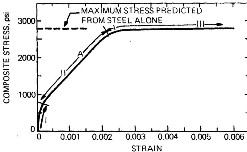
FIGURE 20 The three stages of typical stress-strain curve for ferrocement. (Walkus, I. R. [Lodz Technical Univ., Poland], and T. G. Kowalski [Hong Kong Univ.], "Ferrocement: A Survey." *Concrete* [London]. Vol. 5, No. 1, Feb. 1971)
