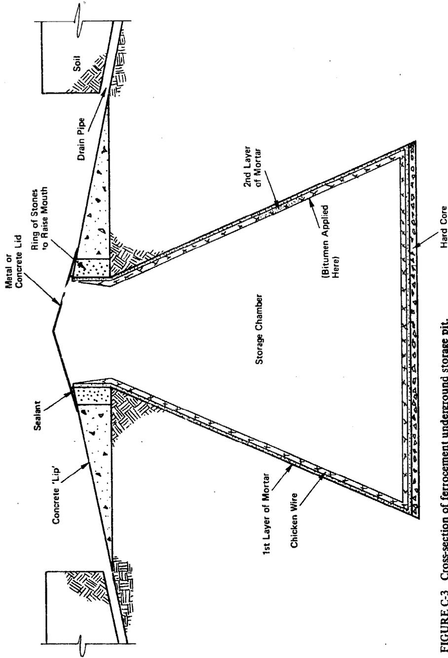
FIGURE C-3 Cross-section of ferrocement underground storage pit.
