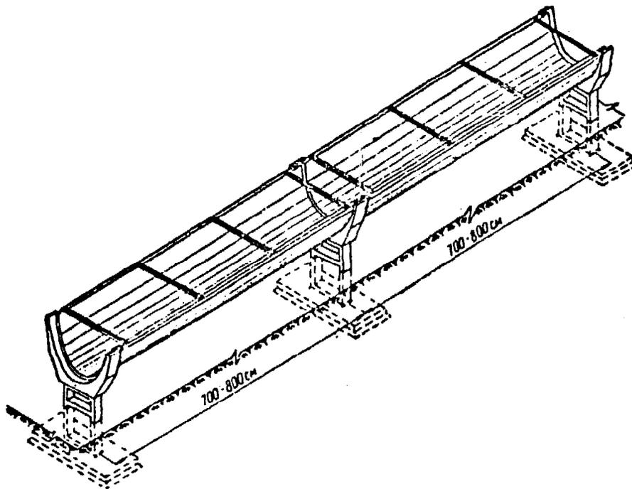
FIGURE 1 Water-conveying troughs, 20 mm thick, are mass-produced in precast ferrocement units in the USSR. (Drawn from diagram in Kowalski, T.G. "Ferrocement in Hong Kong." *Far East Builder*, July 1971, p. 29.)
