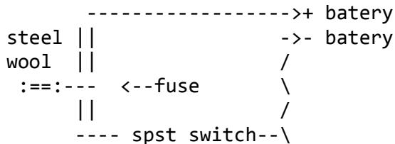
So when the switch is on the currnet will flow through the steel wool or igniter and heat up causing the fuse to light.
