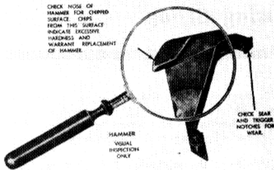
Fig. 147. Points to inspect on hammer.
