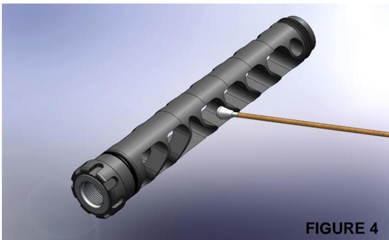
4. Using solvent and a small plastic bristle brush or cotton swab, clean the female threaded socket in the rear of the core assembly. See Figure 5.
