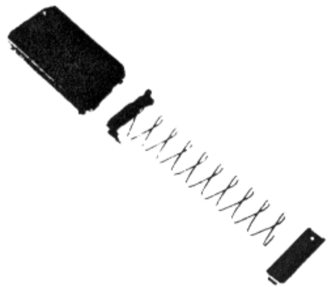
Disassemble/Assemble Magazine Figure 3-19b
