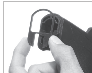
Install the shim between the stock and receiver.
