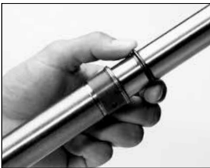
The tapered end of the gas bracket seal must face the gas bracket.
