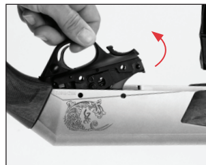
Lift the trigger group from the receiver.
