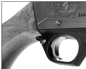
The "safety" shown in the on safe position.
