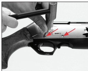
Tap the trigger group pins through the receiver.
