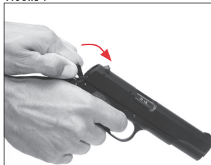
Lowering the hammer to the dropped position.
