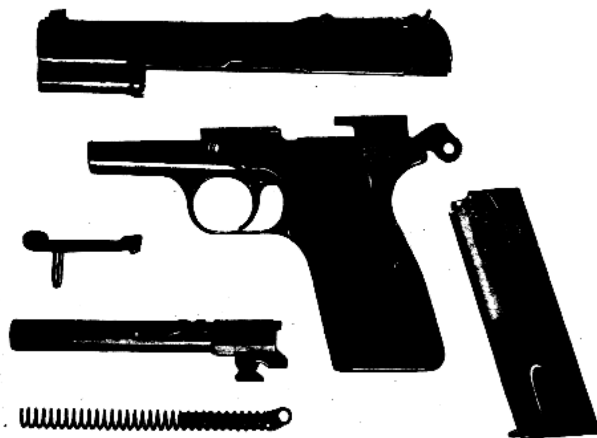
FIGURE 9. Pistol dismantled in main parts
