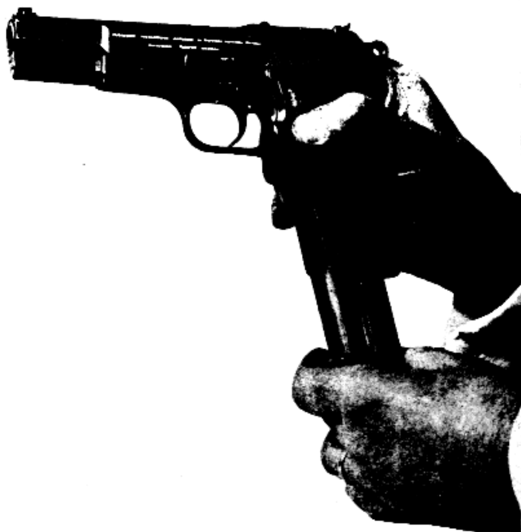
FIGURE 5. Removing the magazine.
