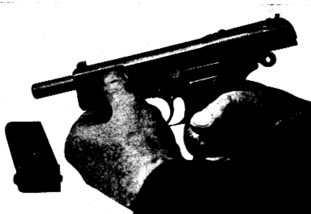
FIGURE 6. Removing the slide stop.
