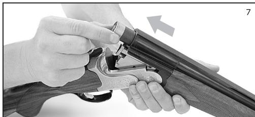
Once the breech is open and the shells removed the gun is safe. Remember to keep the breech open until you are ready to reload to prevent any mistakes or confusion as to the condition of the gun. If the breech is open anyone can see that the gun is unloaded.
