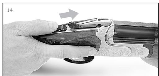
Take the shotgun off safe by pushing the safety forward with the thumb of the shooting hand (figure 14).
