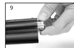
Care should be taken to ensure the keys on the wrench engage in the six large notches in the choke. Hold the gun tightly and unscrew the choke in a counter clockwise direction until it can be removed from the barrel.
