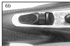
**CAUTION:** Barrel selection should be made while the safety lever is in the safe "S" (on) position.
