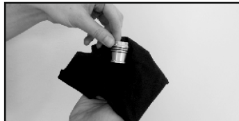
7- Clean the inside and the outside of the piston using the same method.
