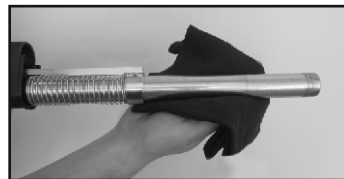
6- Push the latch under the trigger group (Loading figure 2/cartridge drop lever). Pull back the bolt handle. Clean the outer surface of magazine tube with a soft cloth.
