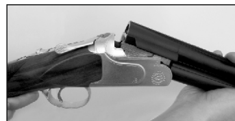
6- By forcing the barrel upwards close the shotgun, be sure the barrel and receiver are properly aligned and top lever returns to slightly to the right of center. It is normal that the top lever does not return exactly to the center, this allows for wear.
