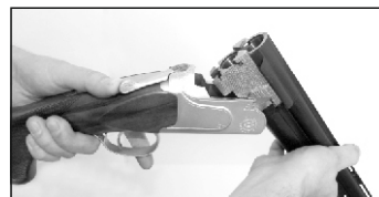
4- While keeping the top lever pushed to right install the barrel to the receiver with an approx 40-degree angle as it is seen in the figure. Be sure the barrel is completely installed to the receiver otherwise shotgun will not close.
