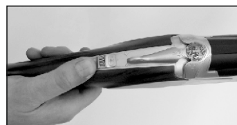
8- Put the safety on by moving the safety switch to the rear position.
