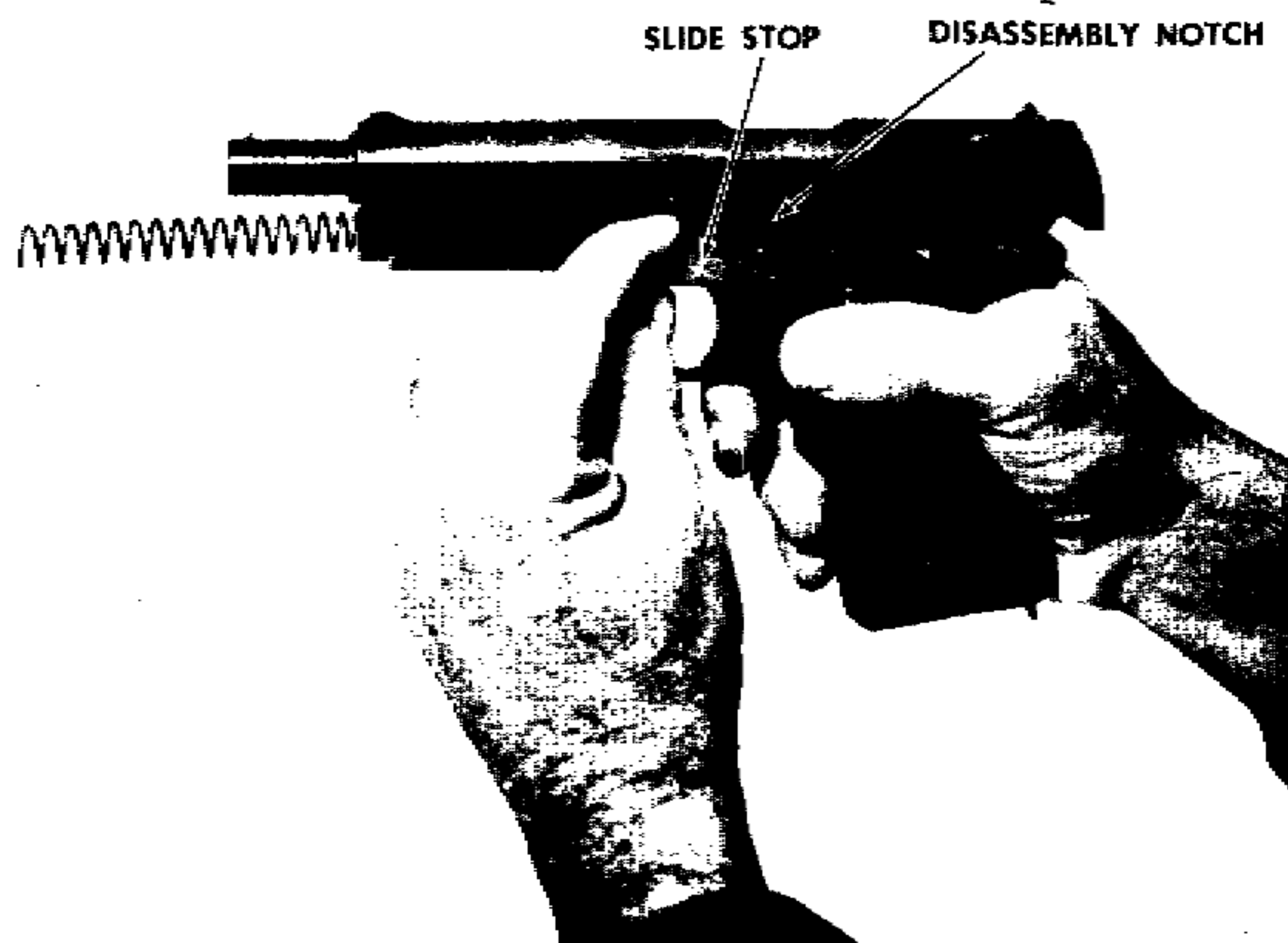
Figure 8. Press the safety lock downward to the FIRE position. Push the slide to the rear until the disassembly notch is aligned with the rear projection on the slide stop. Press the protruding end of the slide stop pin with the right forefinger and pull out the slide stop.
