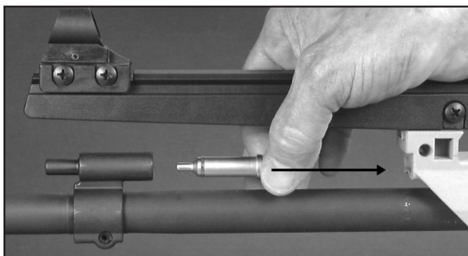
Figure 28 Removing the gas piston
