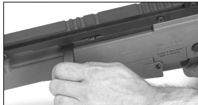
Figure 20 Operating the cocking lever
