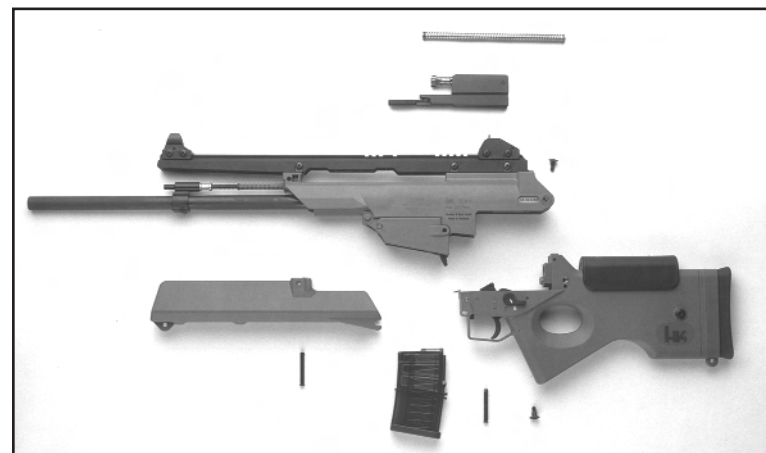
Figure 26 Stripping SL8-1 into assembly groups
