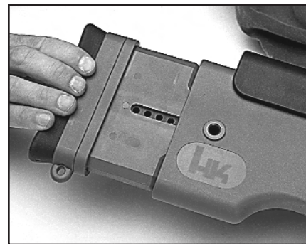
Figure 35 Remove buttplate with spacer
