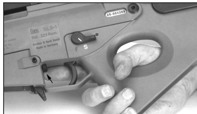
Figure 21 Activate bolt catch, push upwards
