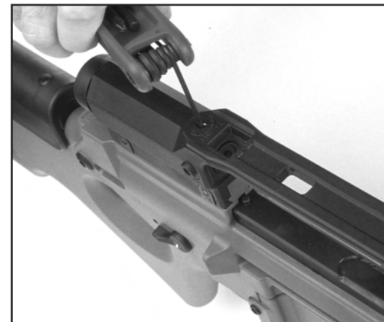
Figure 42 Optical sight elevation adjustment on the SL8-1
