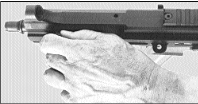
Fig. 24 Pull cocking lever backwards
