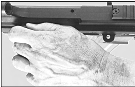
Fig. 20 Pull cocking lever backwards
