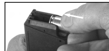
Fig. 17 Filling the magazine
