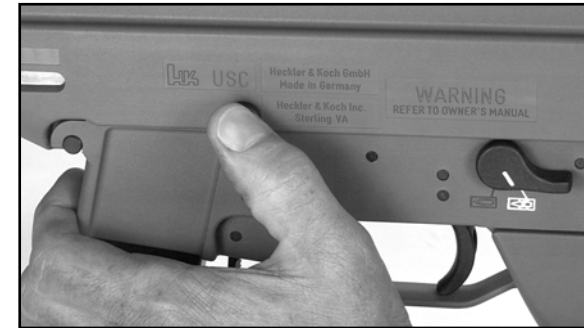
Fig. 21 Depress bolt catch to release the bolt
