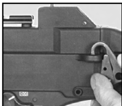
Fig. 34 Attaching carrying sling
