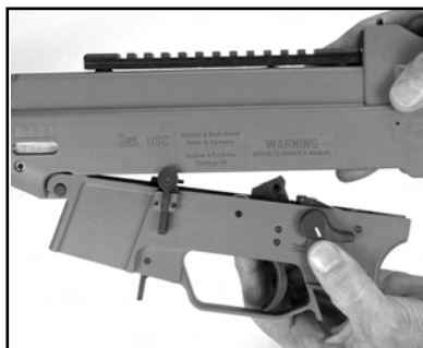
Fig. 23 Detaching lower receiver
