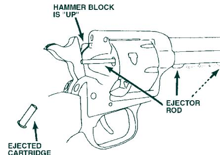
**WARNING: Do not Carry this revolver with a live round chambered under the hammer and firing pin. Keeping an empty chamber under the hammer with the hammer block in the up position is good insurance against accidental firing.**
