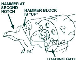
Open loading gate and remove cylinder from right side of gun.
