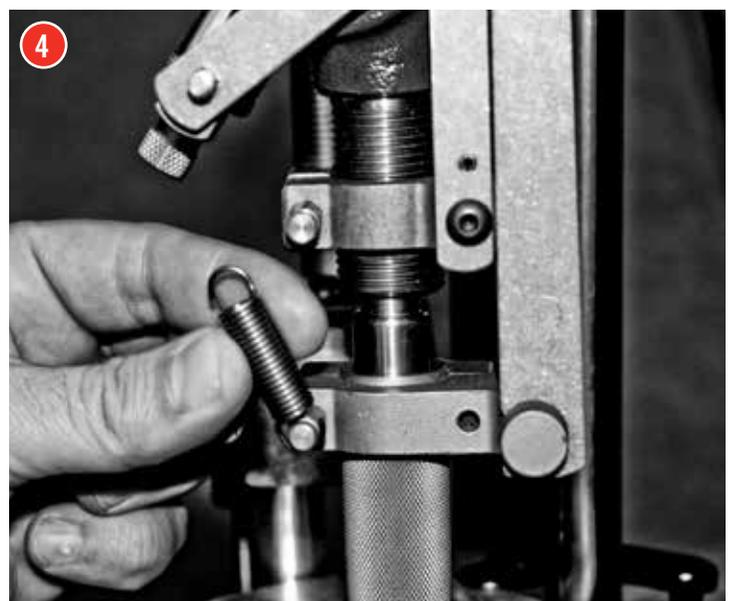
**5** Holding the PTX Powder Measure Stop, unscrew one of the cap screws until the threaded end of the screw is flush with the inside of the slot.
