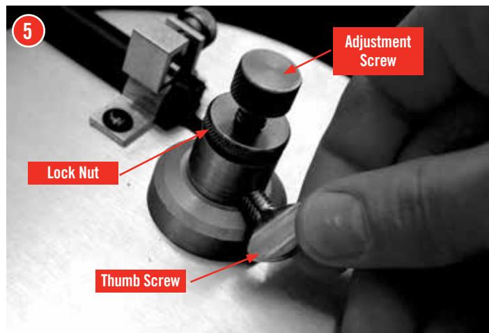
6 Raise the Bullet Guide Plate (11) by turning the Adjustment Screw (6) clockwise far enough to hold a bullet base first against the Bullet Guide Plate (11). You will need to adjust the Bullet Guide Plate up or down to get a bullet to feed base first, but fall off if the bullet is nose first. Tighten the Lock Nut (7) once set.
