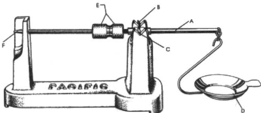
The substitute weight method used in the Pacific Standard Scale is one of the most accurate weighing methods available.
