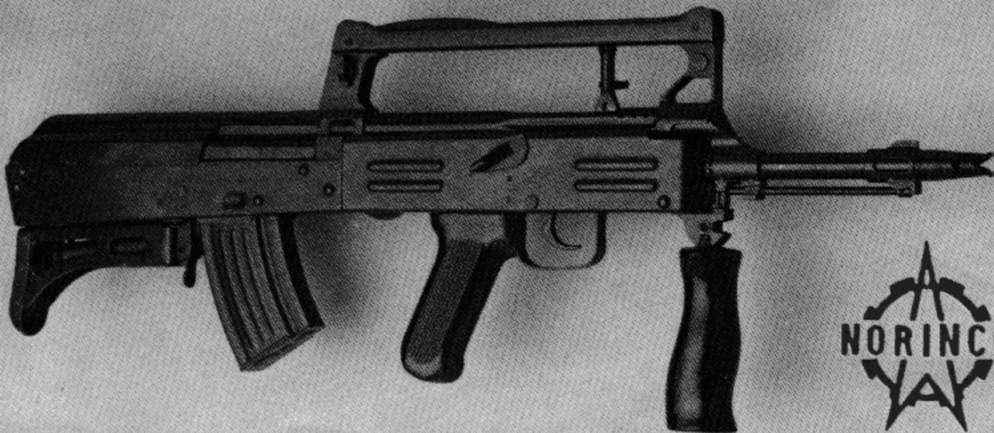
The Type 86S Bullpup operates in the same way as the other AK type rifles with the exception that the cocking handle has been placed on the top of the receiver rather than on the side.
