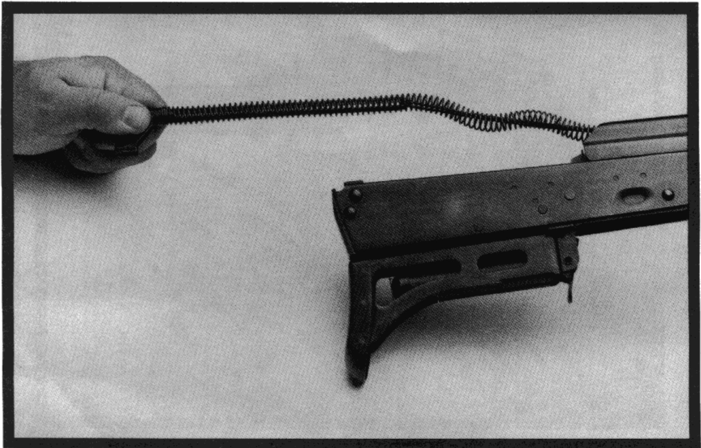
**Slide the recoil spring guide and spring forward out of their notch in the rear of the receiver and remove.**
