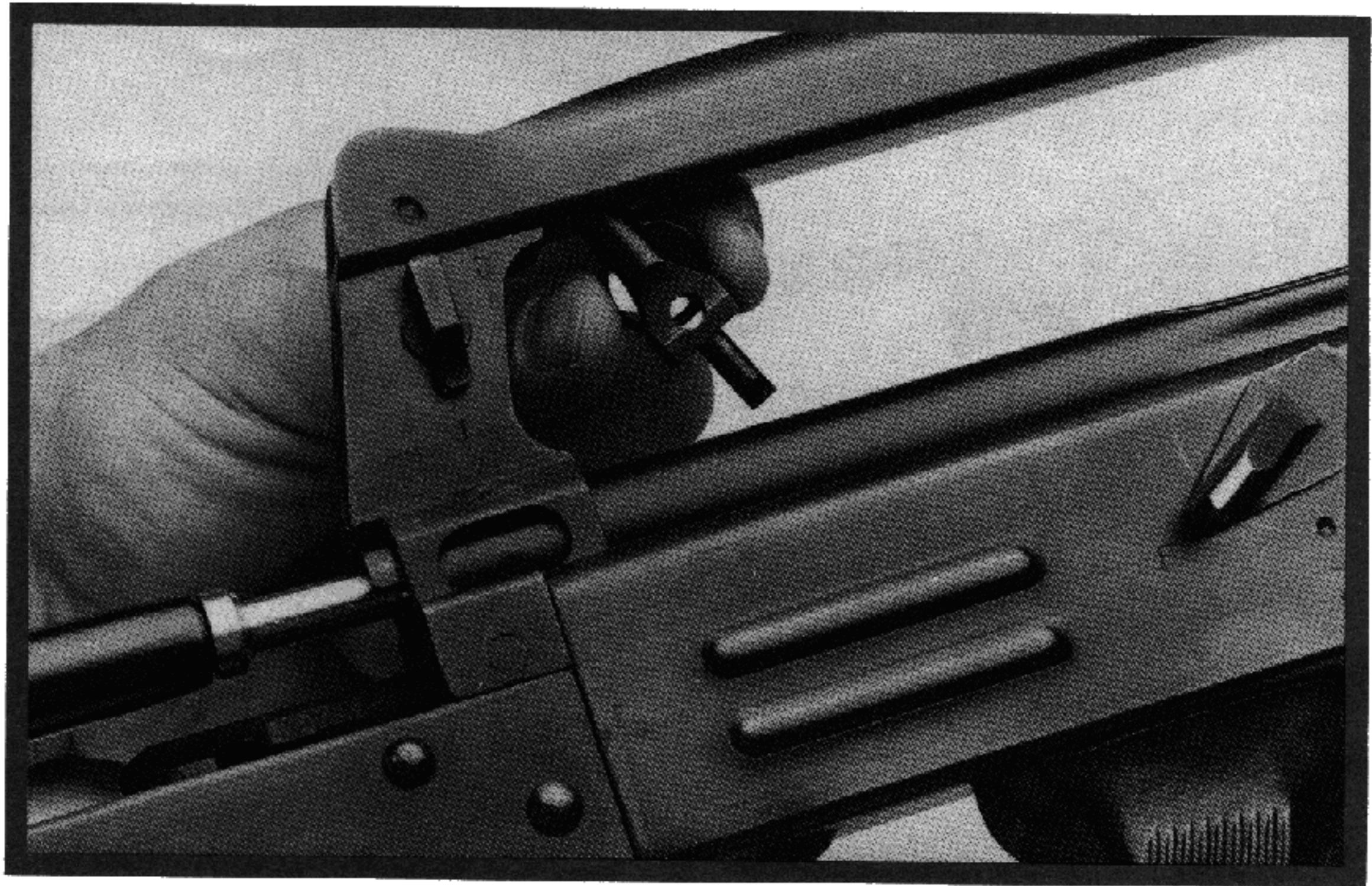
The bolt carrier with its attached piston is now free to slide back and forth. Slide it back until it begins to lift out. At this point the cocking lever will be in line with the hole in the top of the carrying handle. Lift the cocking lever up and out of its notch in the gas piston and remove.
