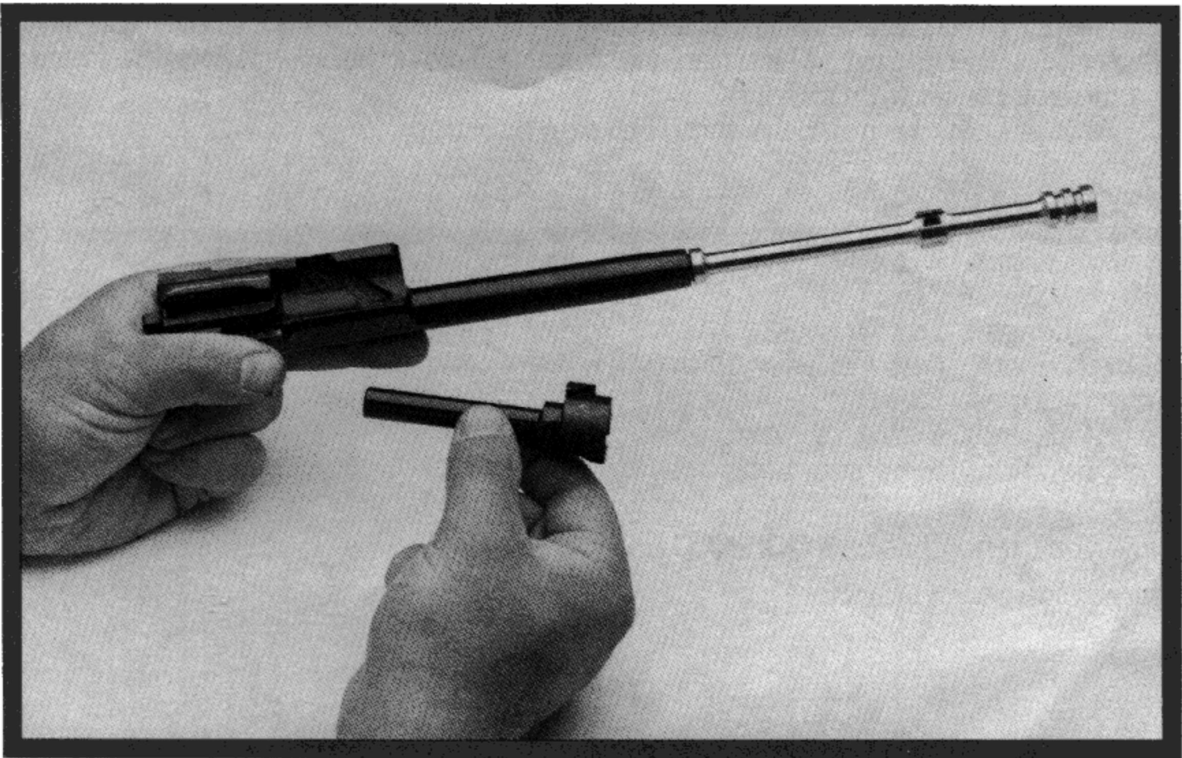
**The bolt is removed from the bolt carrier by turning counterclockwise and pulling forward.**
