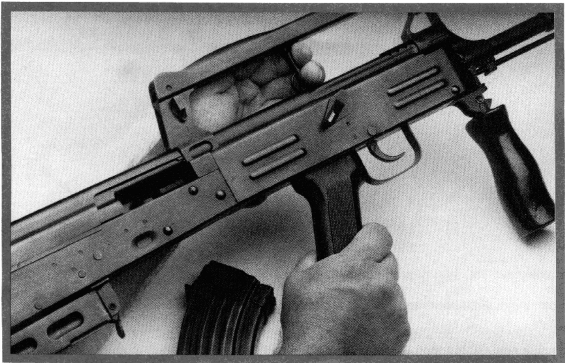
**DISASSEMBLY:** To disassemble the 86S for cleaning and maintenance, first remove the magazine and pull the bolt back to check and see that the chamber is empty and no ammunition is in the rifle.
