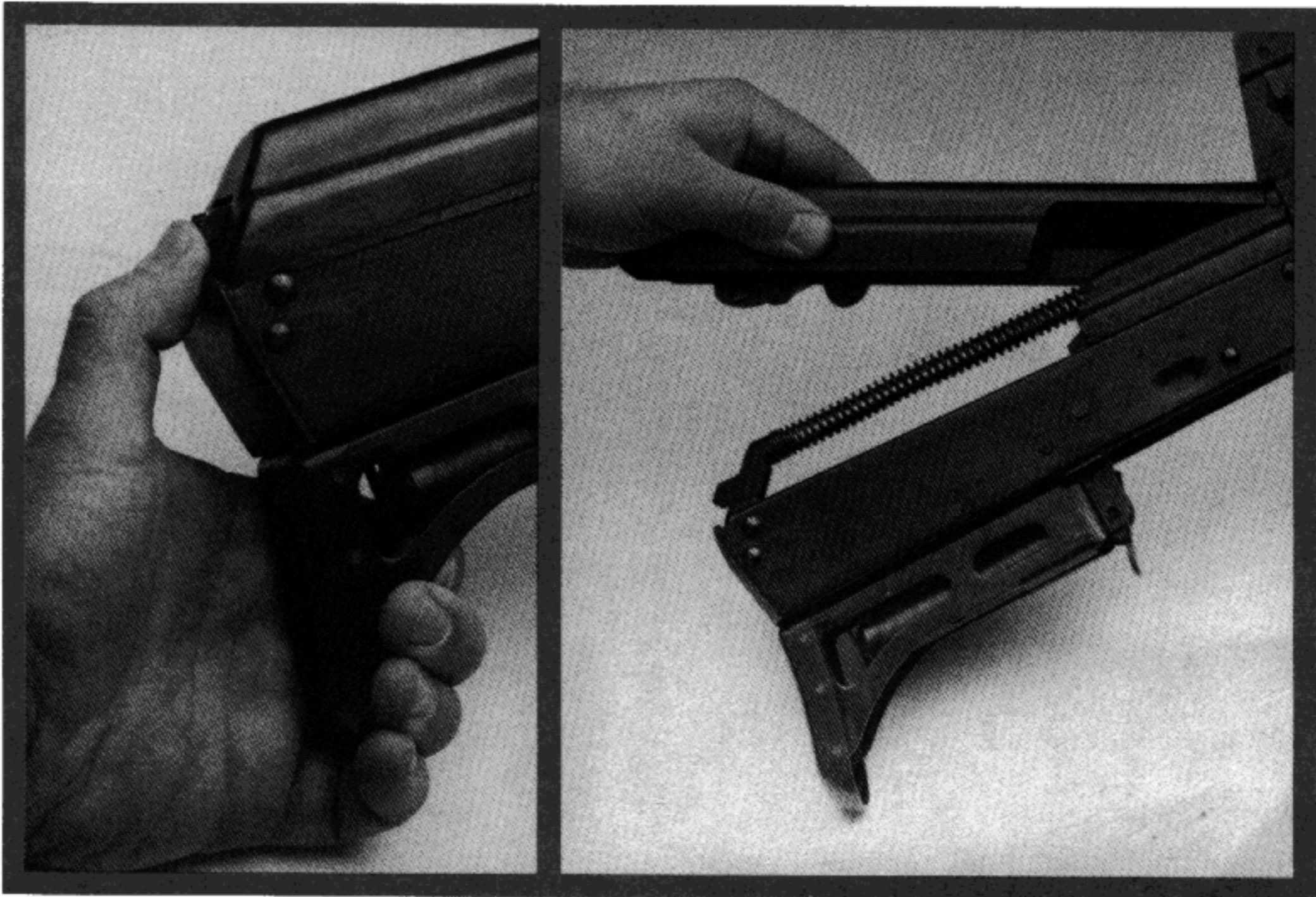
Press in on the latch located at the top rear of the rifle and lift the top cover off.
