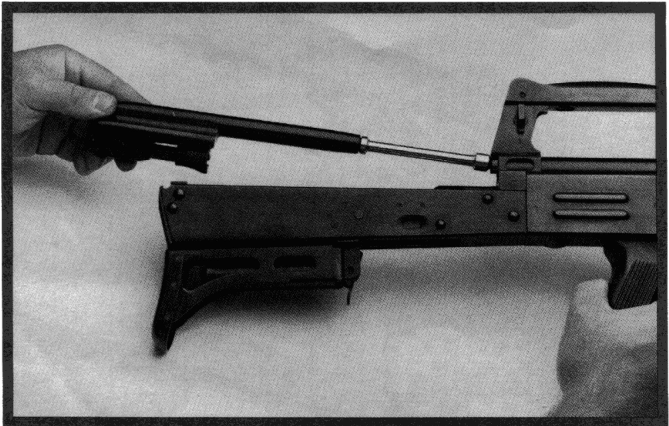
**The bolt and bolt carrier are now free to be removed from the rifle.**
