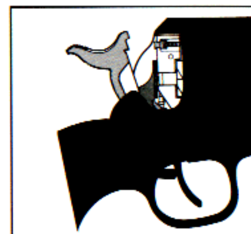
4. Hammer in loading notch position. For loading and unloading only. See “Safe Carrying Position Warning”, p. 11.
