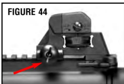
Note: The mounting rail on the top of the pistol will accept any Weaver®-style or Picatinny dimension scope rings or sight base.
