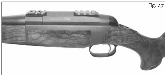
Rail with Picatinny prism (according to Mil. Std 1913)
