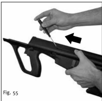
1. Use your right hand to lift the front of the outside ejection lid slightly with a screwdriver while pushing the back of it forward with your left thumb;
