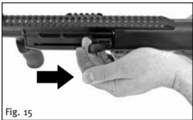
Pull the cocking slide fully back and release it, allowing it to return to the fully forward position.
