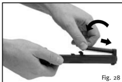
2. Insert the recoil spring into the slide by pressing it down and in.
