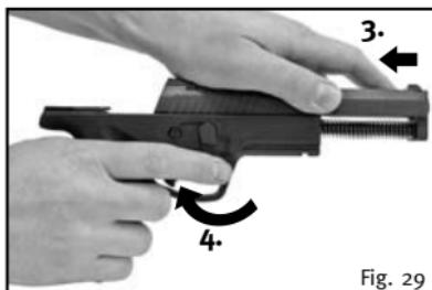
3. Push the slide onto the grip frame towards the back.
