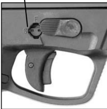
The integrated limited access lock is manually operated by using a separate key. When locked, it locks the trigger and prevents the disassembly of the pistol. The integrated limited access lock can only be locked when the pistol is cocked (trigger in the forward position).
