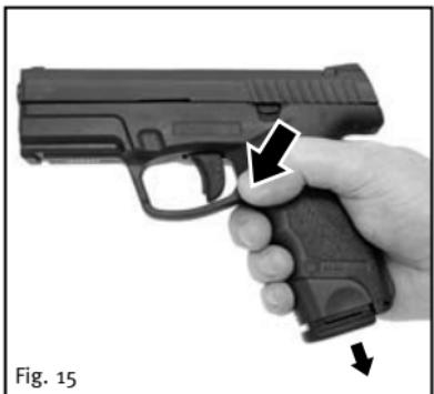
1. Remove the magazine by pressing the magazine release.
