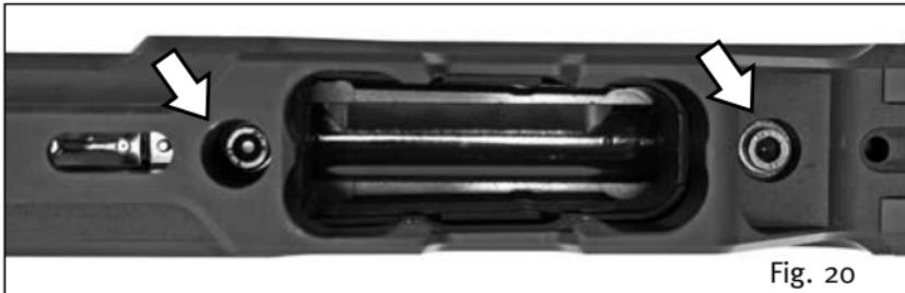
If these screws are loosened, they have to be retightened again with a torque wrench ( $7\text{ Nm}$ ).
