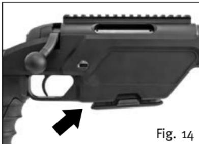
2. Remove magazine or lock it in second position (magazine protrudes by approx. 5 mm/ 0,19").
