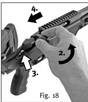
1. Push down the button completely and swing the stock to the left.
