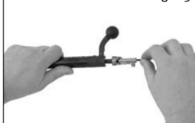
2. Take off bolt sleeve and extract firing pin assembly.
