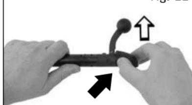
1. Grip the bolt with your left hand. Push in catch lever with your right thumb and simultaneously rotate the bolt sleeve clockwise (arrow shows direction of rotation) until it unlocks with an audible click.
