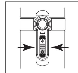
Turn on the LED Flashlight by pushing the ON/OFF switch to center position.
