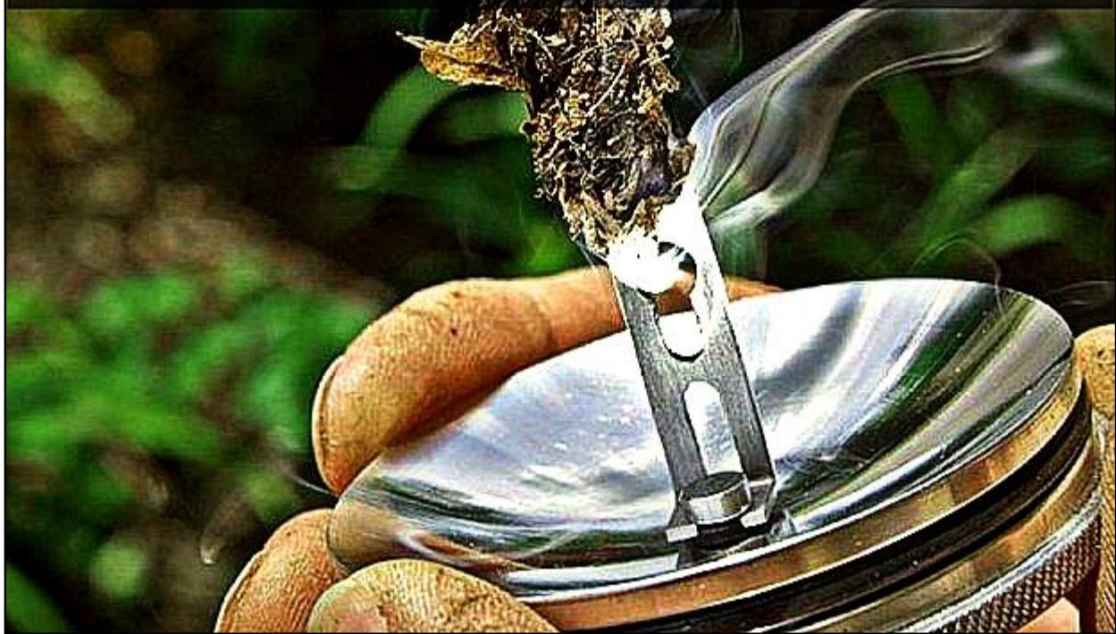
A solar fire starter is basically a magnifying glass that is specifically design to start fires.
