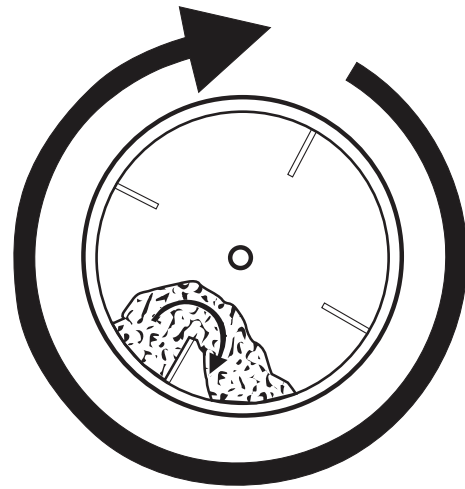
Figure 2. Fin structure in barrel composter.
