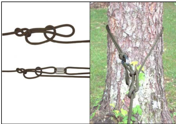
Figure 10-21. TRANSPORT TIGHTENING SYSTEM
