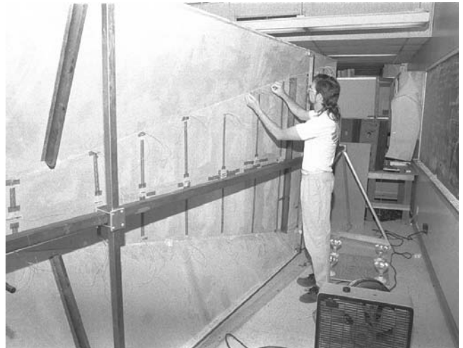
Above: Michael Hackleman routes wires from the diode boards on the back of the PV panel.
