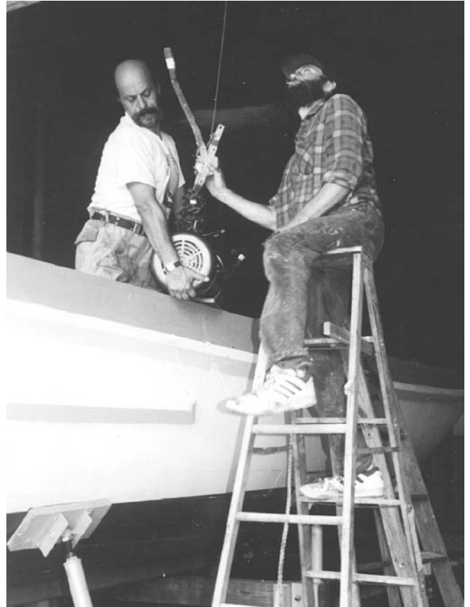
Above: Eighty years after Esther's electric motor was removed, the rotational electron star drive is re-installed.
