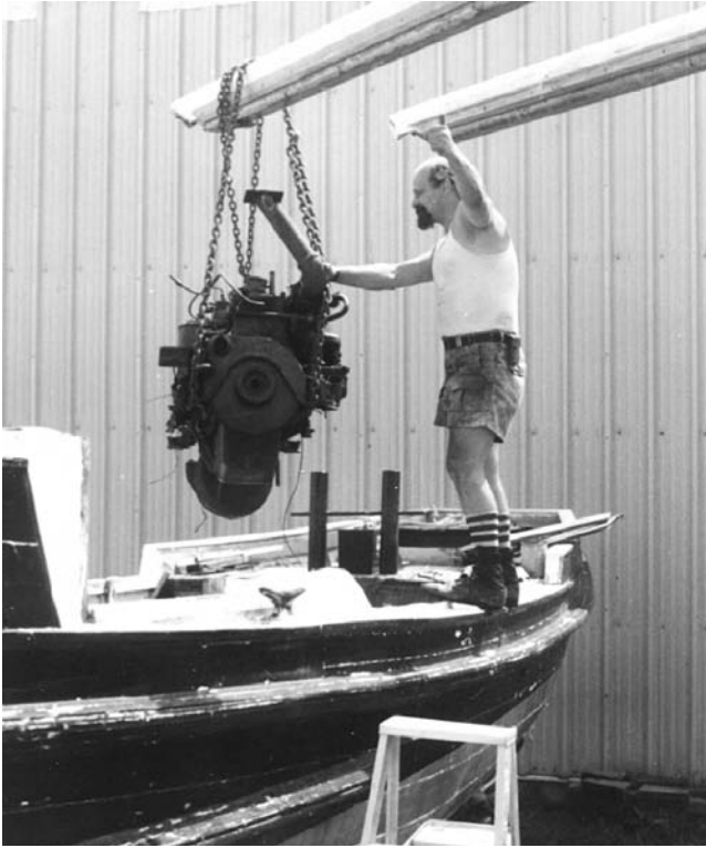
Above: Richard Orawiec removes the Chrysler inline eight remarking, "Beam this INFernal thing outta here...."
