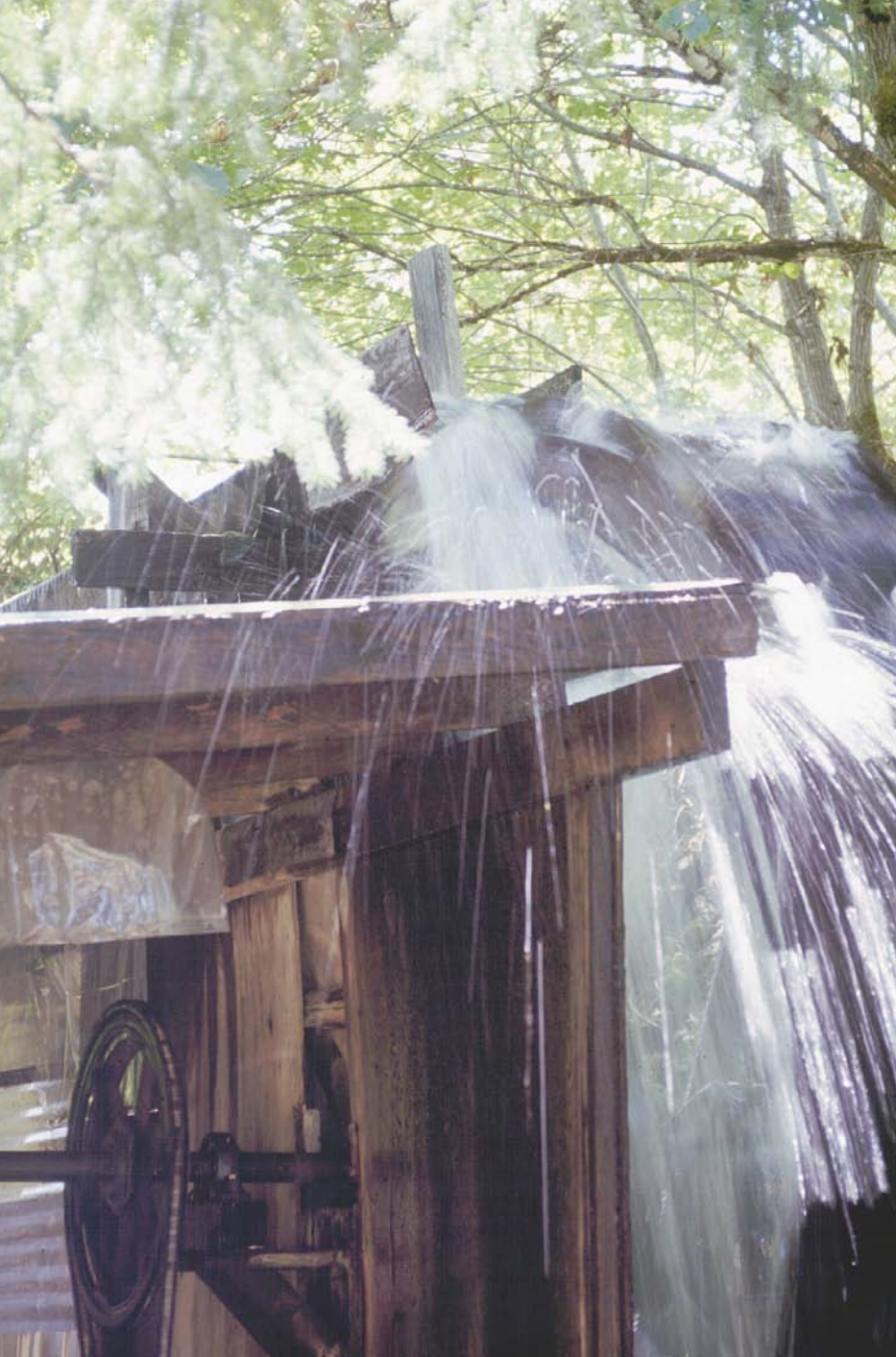
Above: A thirteen foot diameter overshoot hydro wheel makes 2,000 watts of electric power. Photo by Richard Perez
