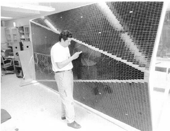
Above: Richard Benevides connects a wire from a bypass diode to a terminator strip on the PV panel.
