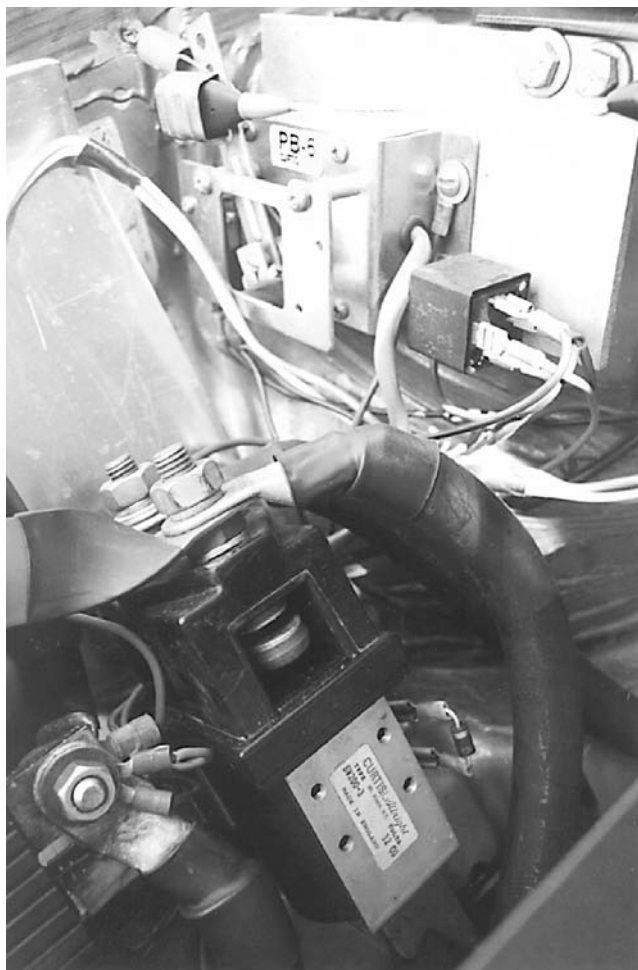
Above: A main contactor is one of the most important safety disconnects. The PB-6 potbox includes a deadman microswitch. Photo by Shari Prange
