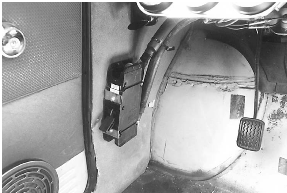
Below: A DC circuit breaker mounted where the driver can reach it quickly. Photo by Shari Prange
