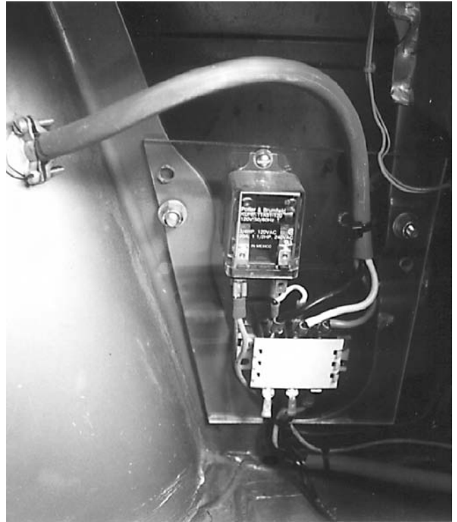
Above: The ac input to the battery charger connects to a relay which disables the vehicle while under recharging. Photo by Shari Prange
