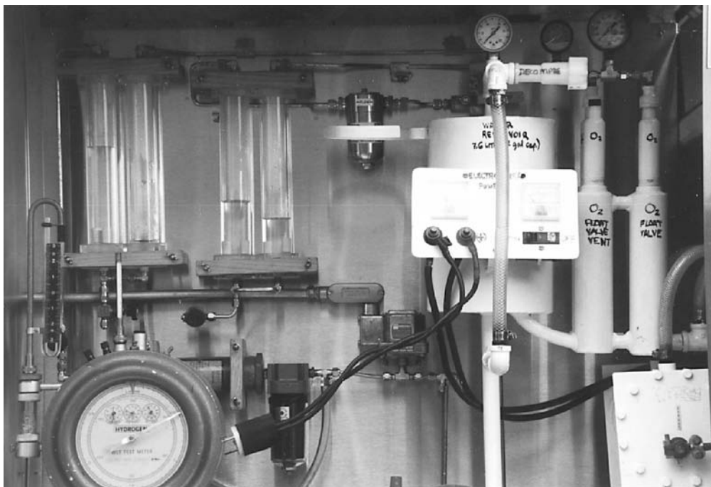
Above: The bi-directional bubblers and purification systems. Photo by Reynaldo Cortez
