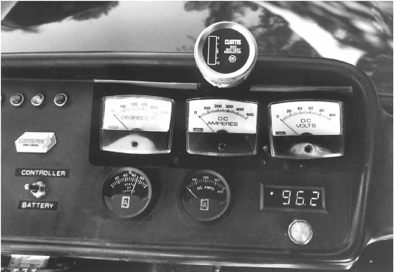
Above: Gauge Styles: LED Bar Scale (top), panel meters (center), automotive (lower left), and LED digital (lower right). Note: leftmost panel meter is sun-faded. Photo by Shari Prange
