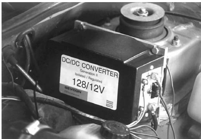
Above: A DC/DC converter installed in a VW Rabbit conversion to keep the 12 volt Accessory battery charged. Photo by Shari Prange
