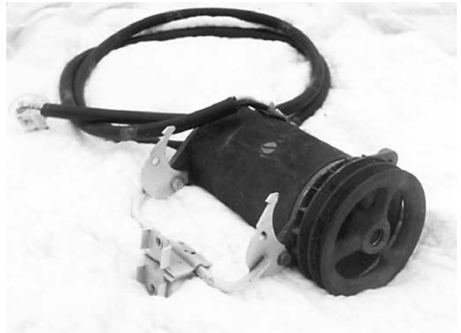
Above: The Delco generator, used as a motor, bolts right on to the Maytag motor mount.
