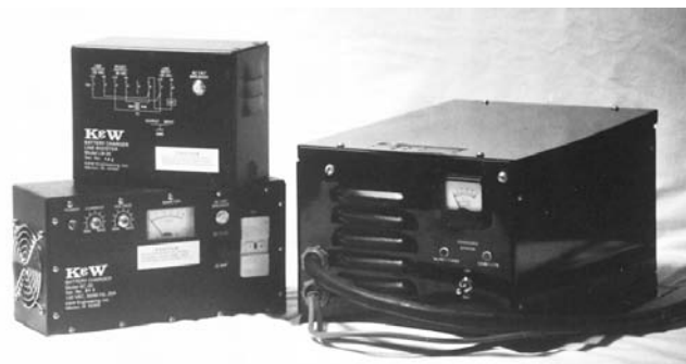
Above: A transformerless 110 volt ac input charger (bottom left); a booster transformer for 120 volt output (top left); and a transformer-type 220 volt input charger (right). Photo by Shari Prange
