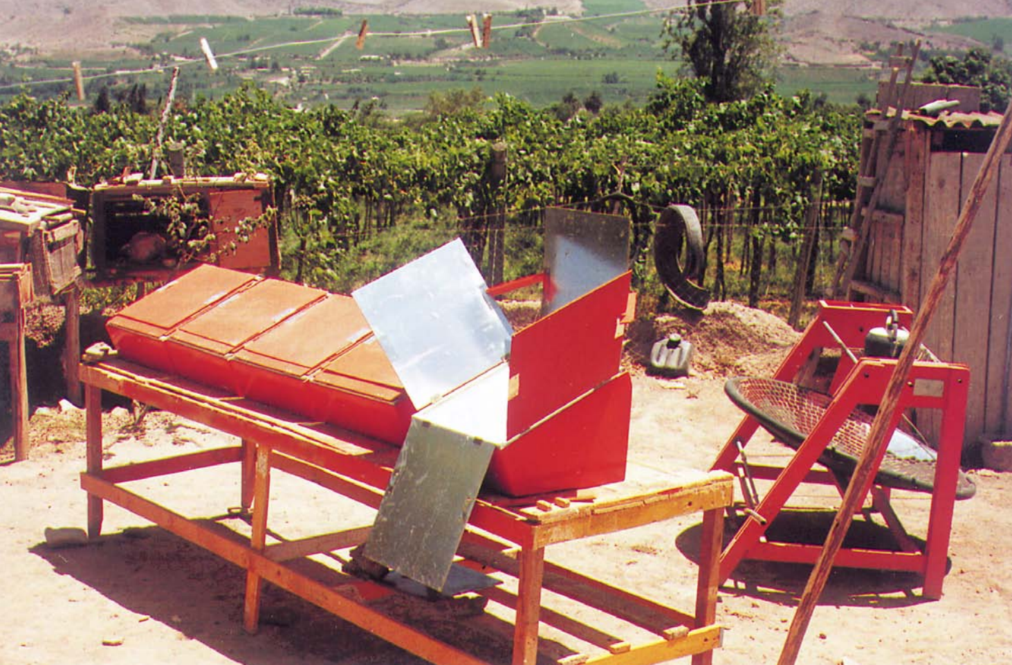
Above: The solar bakery in Villaseca, Chile. The ovens are closed between batches so they won't overheat.
