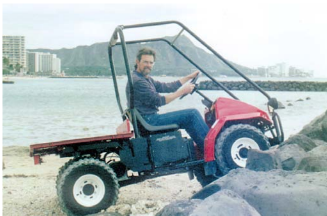
Above: Michael tests the Mule's performance. With the battery pack located so low in the vehicle, this EV felt stable on the rock jettty at the beach.
