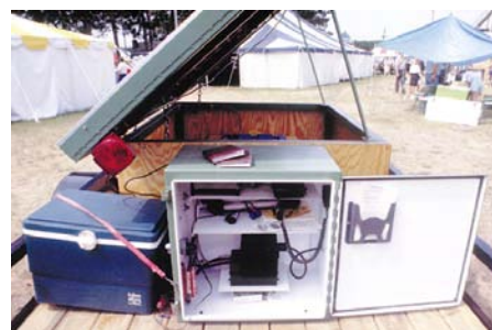
Above left, center and right: Steve Fox of Wyoming, Michigan demonstrates his portable PV power system. This system on a trailer uses eight modules, a 1000 Amp-hr. battery and an Exeltech sine wave inverter. Steve powered seven solid hours of live electric music with this system last Earth Day. The workmanship is first class!
