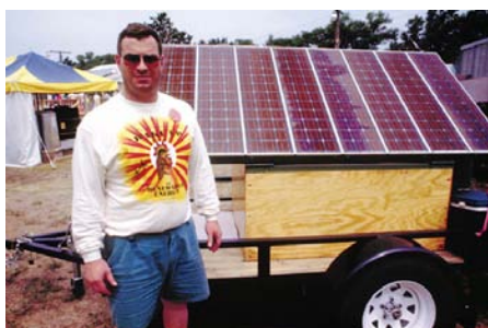
Above left, center and right: Steve Fox of Wyoming, Michigan demonstrates his portable PV power system. This system on a trailer uses eight modules, a 1000 Amp-hr. battery and an Exeltech sine wave inverter. Steve powered seven solid hours of live electric music with this system last Earth Day. The workmanship is first class!
