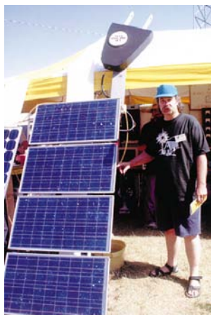
Above left, center and right: Steve Fox of Wyoming, Michigan demonstrates his portable PV power system. This system on a trailer uses eight modules, a 1000 Amp-hr. battery and an Exeltech sine wave inverter. Steve powered seven solid hours of live electric music with this system last Earth Day. The workmanship is first class!
