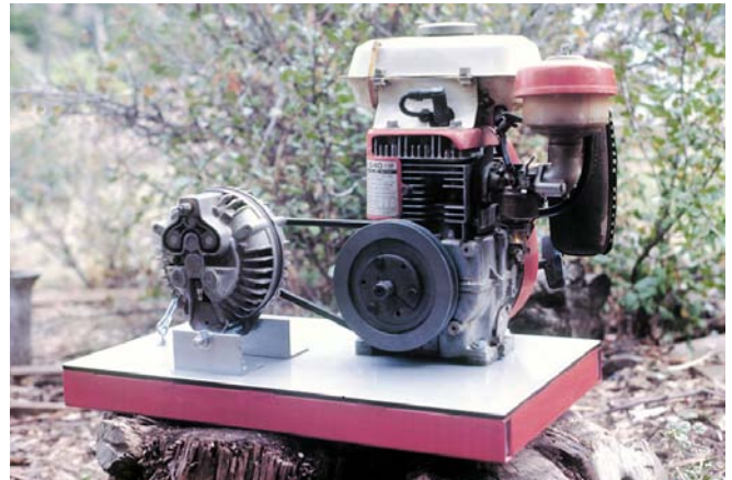
Above: This engine/generator uses a Chrysler 70 Ampere alternator.
