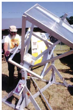
Above left, center and right: Steve Fox of Wyoming, Michigan demonstrates his portable PV power system. This system on a trailer uses eight modules, a 1000 Amp-hr. battery and an Exeltech sine wave inverter. Steve powered seven solid hours of live electric music with this system last Earth Day. The workmanship is first class!
