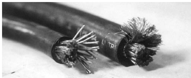
Above: Both regular 2/0 cable (left) and welding cable (right) contain the same amount of copper, but the welding cable is much more flexible. Photo by Shari Prange
