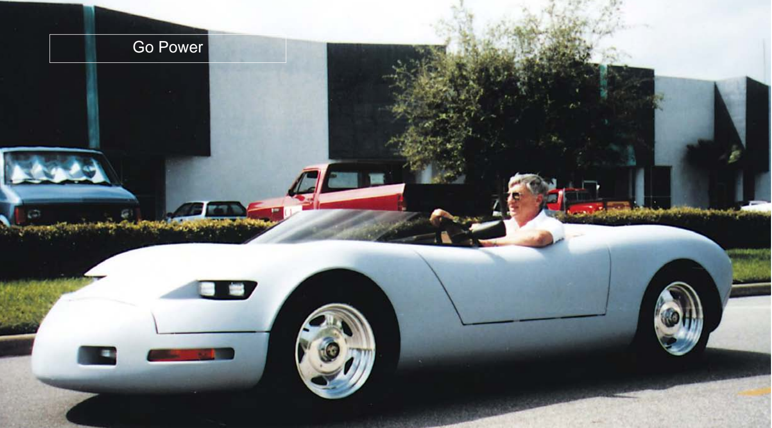
Above: The Tropica, a sporty coupe designed from the ground up to be an EV, has an ABS body, twin EV drivetrains, and an estimated $12,000 price tag. Photo courtesy of Renaissance Cars
