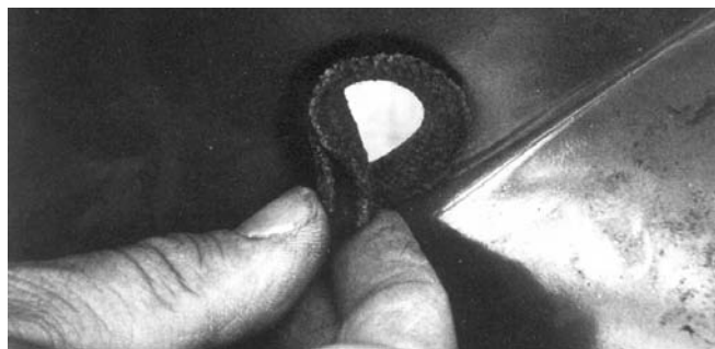
Above: A custom grommet can be easily made from a length of VW fuel line that is slit along one side
