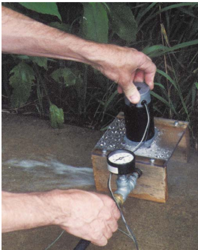
Above: This micro hydro turbine is producing 40 Watts from a garden hose.
