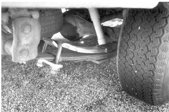
Above: Helper leaf springs beefed up the suspension of this Datsun pickup truck.
