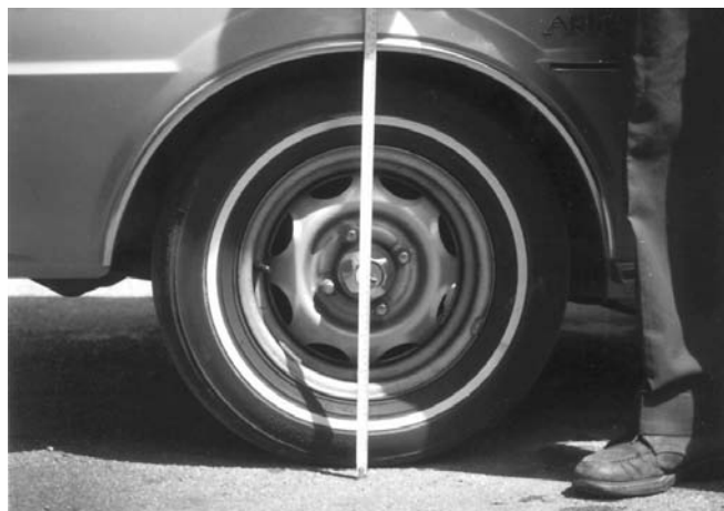
Above: Ride height is measured through the center of the wheel, from the ground up to the wheel arch.
